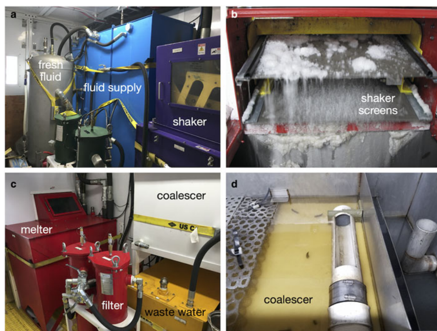
Fig. 5. Photographs showing key components of the FRS. (a) Cold side of the FRS module, showing supply tanks (blue) and primary borehole staging tank (silver). (b) Vibrating shaker consisting of two overlying screens operated by means of an eccentric belt drive. (c) Melting tank inside the warm room, containing a submerged glycol-loop manifold connected to a diesel boiler. (d) Coalescing tank containing baffles and a weir that drains ESTISOL™ 140 floating on water.
