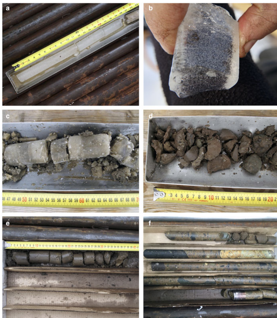
Fig. 10. Photographs of cored materials recovered in hole 2. (a) Dirty glacial ice below 677 m with flecks of rock debris. (b) Close-up of glacial ice containing air bubbles. (c) Dirty, banded ice from ~678 m. (d) Soft, gritty till containing pebbles. (e) Hard, dry, compacted till (surface is wet from drilling fluid). (f) Bedrock core of heterolithic tillite from ~679–681 m. Measuring tape in cm.
