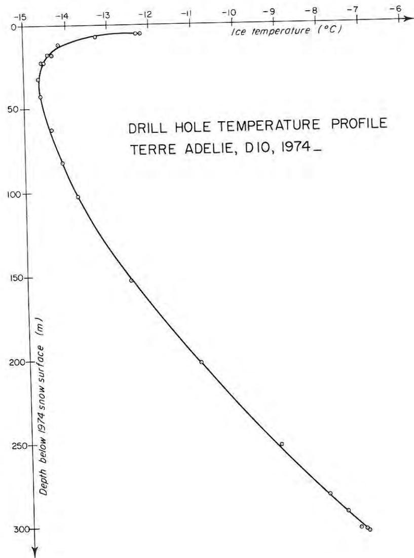
Figure 3. Drill hole temperature profile, Adélie Coast, Antarctica, January 1974. (Data obtained by Claude Rado.)
