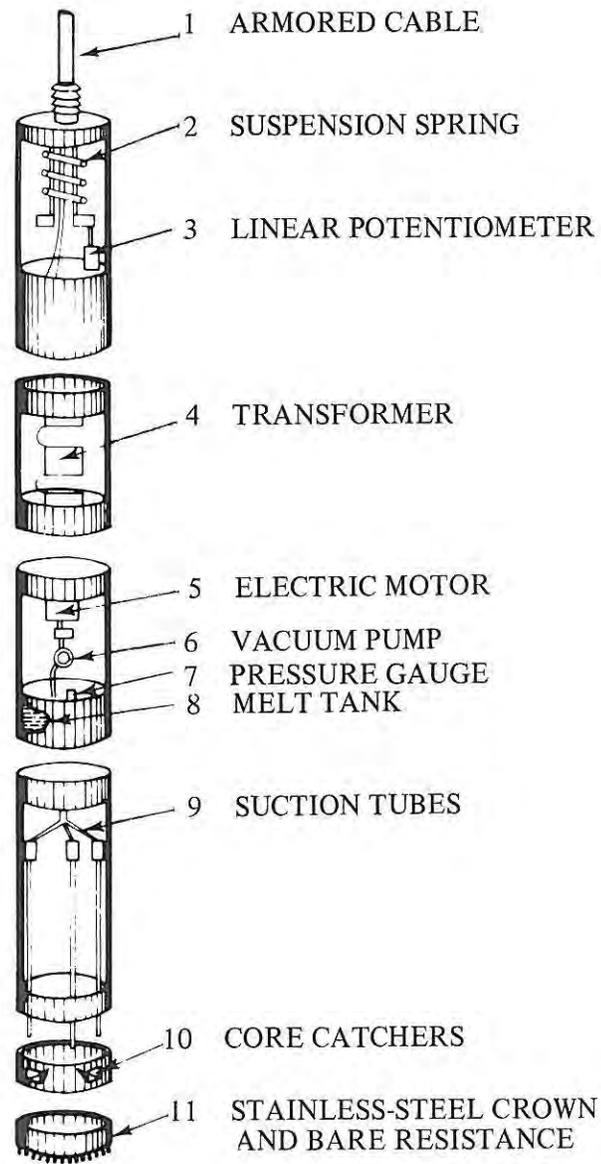
Figure 1. Diagrammatic sketch of corer.
