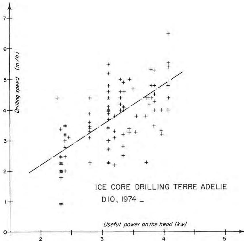
Figure 4. Speeds obtained in ice drilling, Adélie Coast, Antarctica, January 1974.
