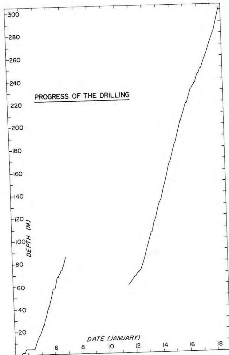
Figure 2. Progress of drilling, Adélie Coast, Antarctica, 1974.
