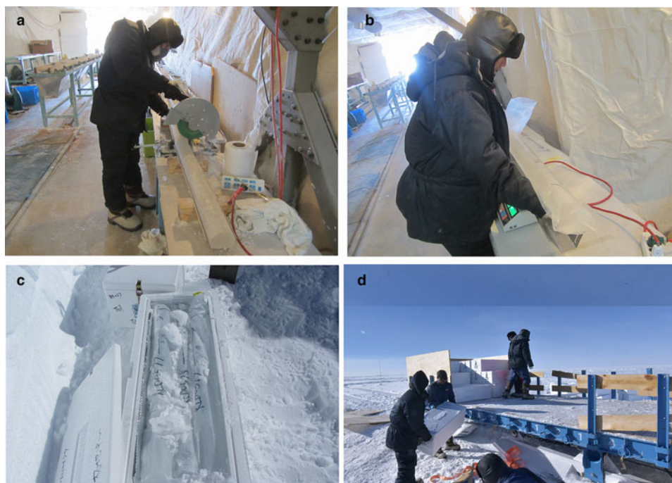
Fig. 6. (a) Cutting the ice core to length; (b) weighing the ice core; (c) packing the ice core into the insulated transport box; and (d) stowing boxes on a sled for transportation.
