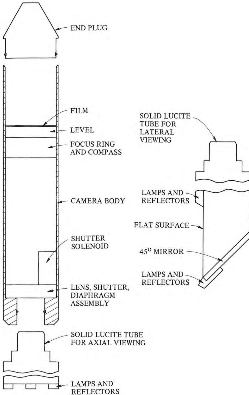
Figure 2. Borehole camera including tube for axial viewing at left; tube for lateral viewing at right. The outside diameter of the camera is 51 mm.
