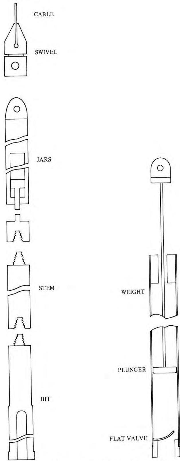
Figure 1. Cable tool (left) and sand pump (right). The bit, stem, and jars are respectively about 0.6, 2.0 and 0.5 m long; the maximum diameter of the bit is about 50 mm. The body of the sand pump is about 1.5 m long and 51 mm in diameter.
