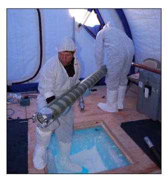
**Prairie Dog** – A modification of the hand auger, the Prairie Dog includes a stationary outer barrel that allows operations in solid ice as well as firn. Limit of depth of use is approximately 40 meters (with a Sidewinder). The drill has been used almost exclusively by Jay Kyne, its designer, who is now a contract driller with IDDO.
