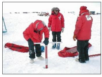
or half-meter cores. The maximum depth to which hand augers without power assistance (see section on Sidewinder) can be used is approximately 20 meters.
