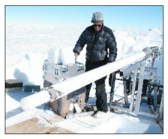
Badger-Eclipse Drills – The Badger-Eclipse Drills are modified Eclipse Drills manufactured by Icefield Instruments, Inc. The drill is electromechanical and takes an 81 mm core to depths of approximately 400 meters. The drill system is transportable by small aircraft or helicopter. There has been an increased demand for use of the drills on field projects and a third Eclipse Drill has been transferred from the University of New Hampshire to IDDO.
