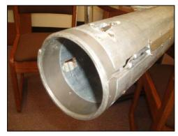
Electrothermal Drill – This drill melts an annulus around the core. It supplements the 4-Inch drills and can be substituted for the 4-Inch sonde, using the same winching system, for use in ice warmer than about minus 10° C. It takes a 3-inch core. It is particularly useful in ice close to the pressure melting point, where electromechanical drills suffer risk from melting and refreezing of the ice. Much simpler than the electromechanical drills, the electrothermal drill
