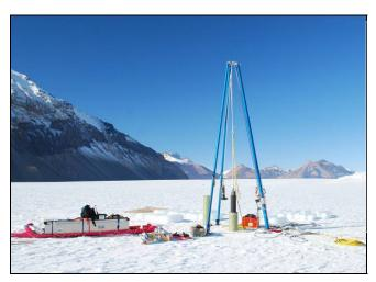
Blue Ice Drill –An agile drill capable of retrieving cores of approximately 9 1/2 inch diameter to depths up to 20 meters in solid ice. The drill, developed for the University of California at San Diego, was used with great success to collect samples of "blue ice" on Taylor Glacier during the 2010-11 Antarctic field season.
