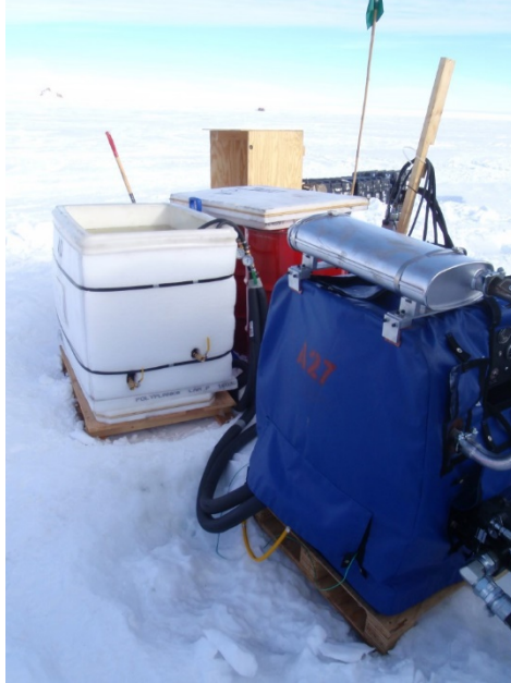
Figure 3: 8kW, 50 gallon capacity chip melter system (white tank) using waste heat from one of the Agile Sub-Ice Geological (ASIG) Drill diesel engines (under blue cover) to melt and separate cuttings from the drilling fluid
