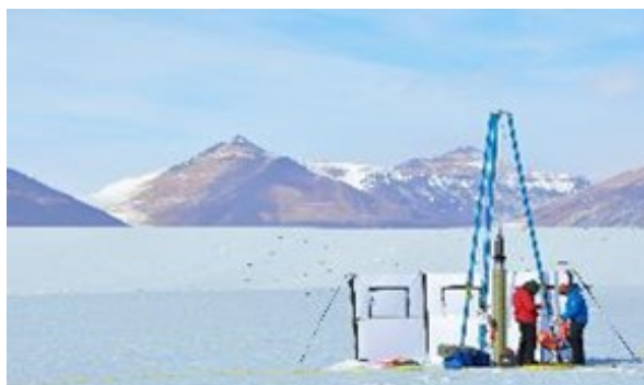
A large-volume ice core drilled on the Taylor Glacier ablation zone, Antarctica. Bubbles in the ice at the site contain air with direct evidence of ancient atmospheric composition. The Blue Ice Drill is an easily-transportable drill capable of retrieving quality firn cores of approximately 9.5 inches in diameter as well as quality solid ice cores of the same diameter with few cracks up to 70 meters below the firn-ice transition. Photo credit: Jeff Severinghaus .
