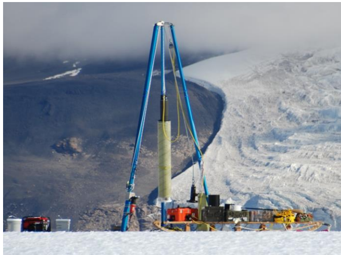
The Blue Ice Drill deployed in Taylor Valley, Antarctica. The very popular system drills a 9.5-inch diameter core, primarily for onsite melting and gas analysis.
