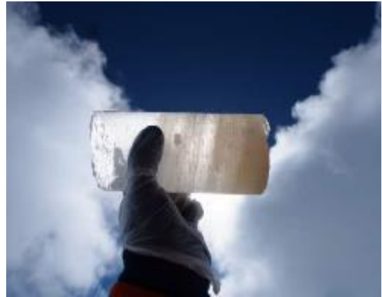
Part of an ice core retrieved from Mt Hunter Plateau of Denali exhibits layering and dust carried to the area from afar. Photo credit: Brad Markle, Univ. Washington
