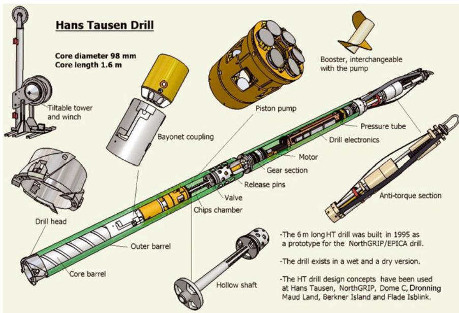
**Fig. 3.** The major components of the HT drill. The first version, a prototype for the deep NorthGRIP and EPICA drills, was tested on Hans Tausen Ice Cap in 1995; it did not have the pump or the bayonet coupling installed. See text for further explanation.
