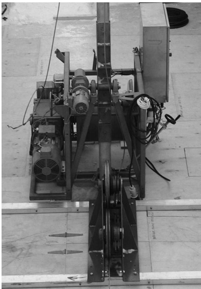
**Fig. 7.** The winch and mast system with cable-tensioning device in the foreground, ready to roll cable onto Lebus drum, visible at the rear of the frame. On the left of the winch frame is the motor and gear reducer; on the right is the handle for engaging the locking mechanism for the mast in the upright position and the winch control panel; in the top centre of the frame is the mast tilt mechanism with its gear motor.
