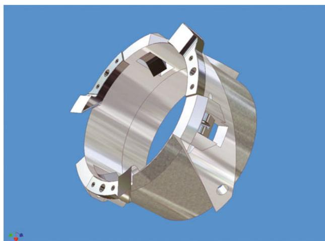
**Fig. 4.** The 4 in (10.16 cm) Hans Tausen drill head is blown up from the one used in the 3 in UCPH shallow drill. The shoes (not shown) that control the pitch are located right behind the cutters for best results. The wet and dry version are slightly different, cutting 129.6 mm and 126.0 mm holes respectively and 98 mm core in both cases. The cutter widths are thus 15.8 mm for the wet and 14.0 mm for dry head. The cutters normally used have a relief angle of 15° and a cutting angle of 45°.
