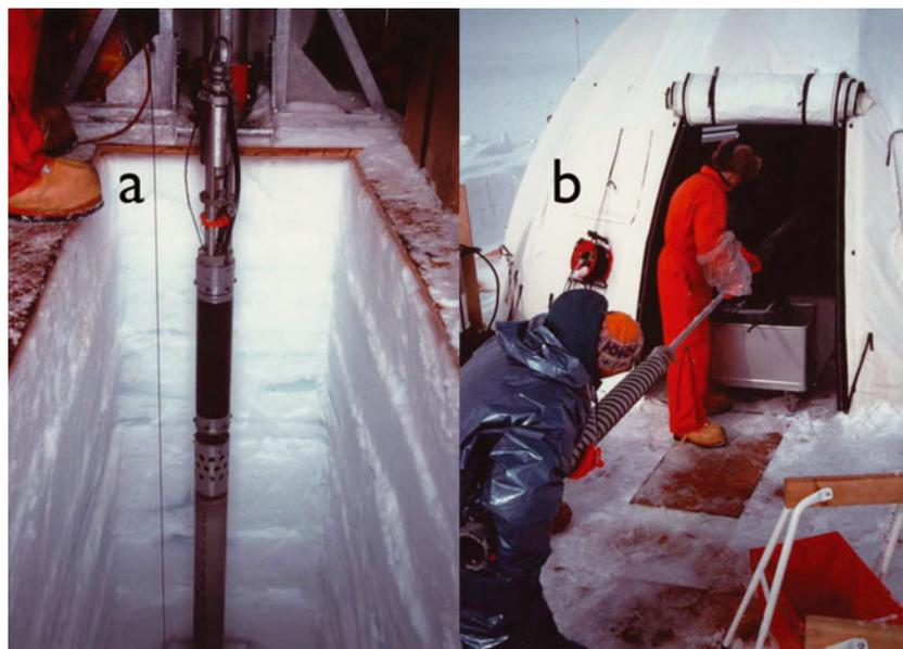
**Fig. 6.** Hans Tausen 1995 drill test. (a) The drill hangs in the drill pit from the shallow winch and tower unit. The base of the winch is seen at top, and the drill parts from top are anti-torque section, (short) motor section and top of chips chamber. (b) S.B.H and P.J. mount the core barrel and hollow shaft inside the drill. When this unit is pulled out, all the chips in the chips chamber will follow, with the top valve acting as piston. The rest of the drill is inside the white dome tent.
