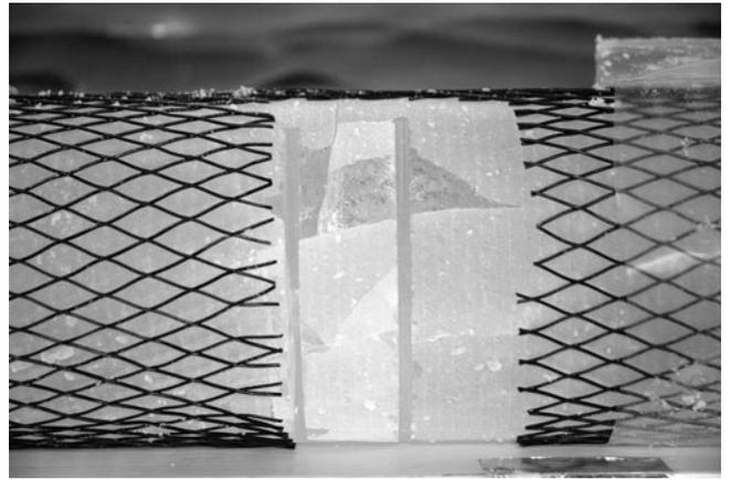
**Fig. 12.** Elastic netting used to contain brittle ice: this core from 920 m has been partially cut with the circular saw shortly after drilling in order to take a subsample, and shows the limited extent of damage to the 'brittle ice'.
