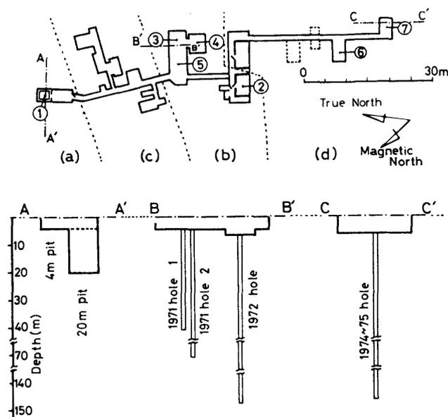
Fig. 2. Plan of Mizuho Station as of January 1975 and vertical sections of the drilling sites and the 20-m pit; ① Refuge hut, ② Living quarters, ③ Drilling site, ④ Glaciological laboratory, ⑤ Generator-site, ⑥ New generator-site, ⑦ New drilling site, (a), (b), (c) and (d) indicate the areas constructed by JARE-11, -12, -13 and -15, respectively.
