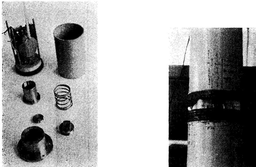
Fig. 12. JARE 140 Mk II: Suspension and pump (left), connection between tank and barrel (right).
