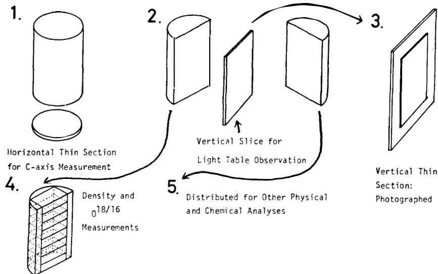
Fig. 8. Cut of JARE-13 cores.
