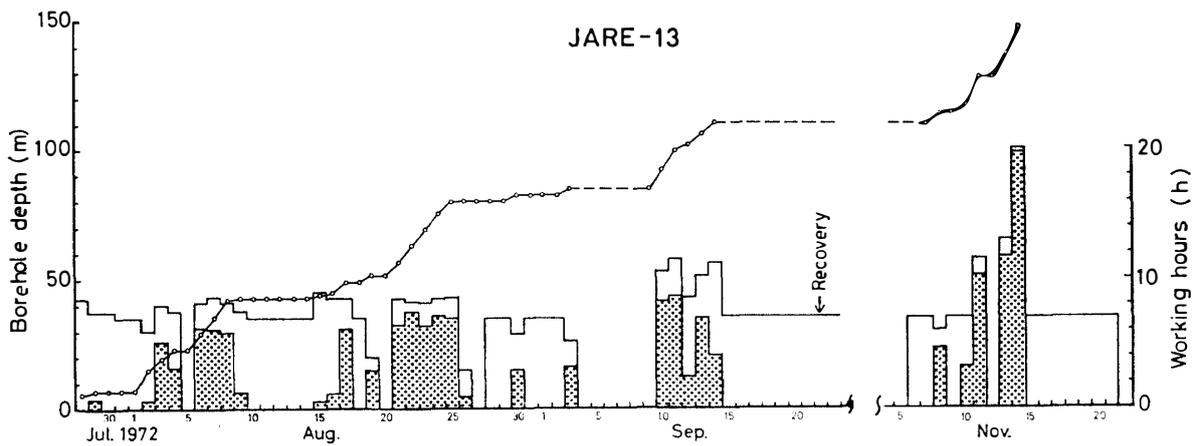
Fig. 5. Progress diagram of drilling in 1972: Dotted area indicates the actual drilling hours and blank area the hours spent for maintenance.
