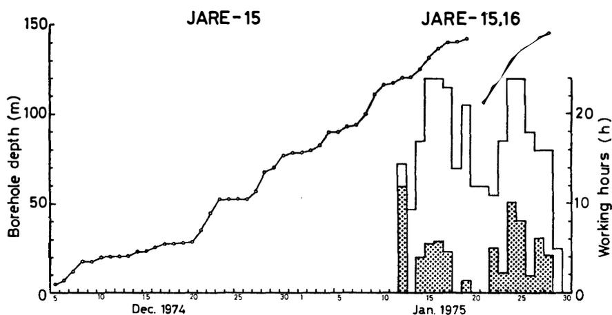
Fig. 6. Progress diagram of drilling in 1974-75: Dotted area indicates the actual drilling hours and blank area the hours spent for maintenance.
