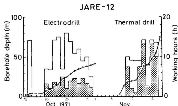
Fig. 3. Progress diagram of drilling in 1971: Dotted area indicates the actual drilling hours and blank area the hours spent for maintenance.
