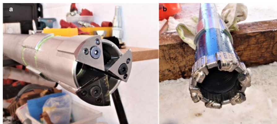
Fig. 5. (a) Full face ice bit and lower reaming shell for drilling the access hole. (b) PDC coring bit for ice and rock.
