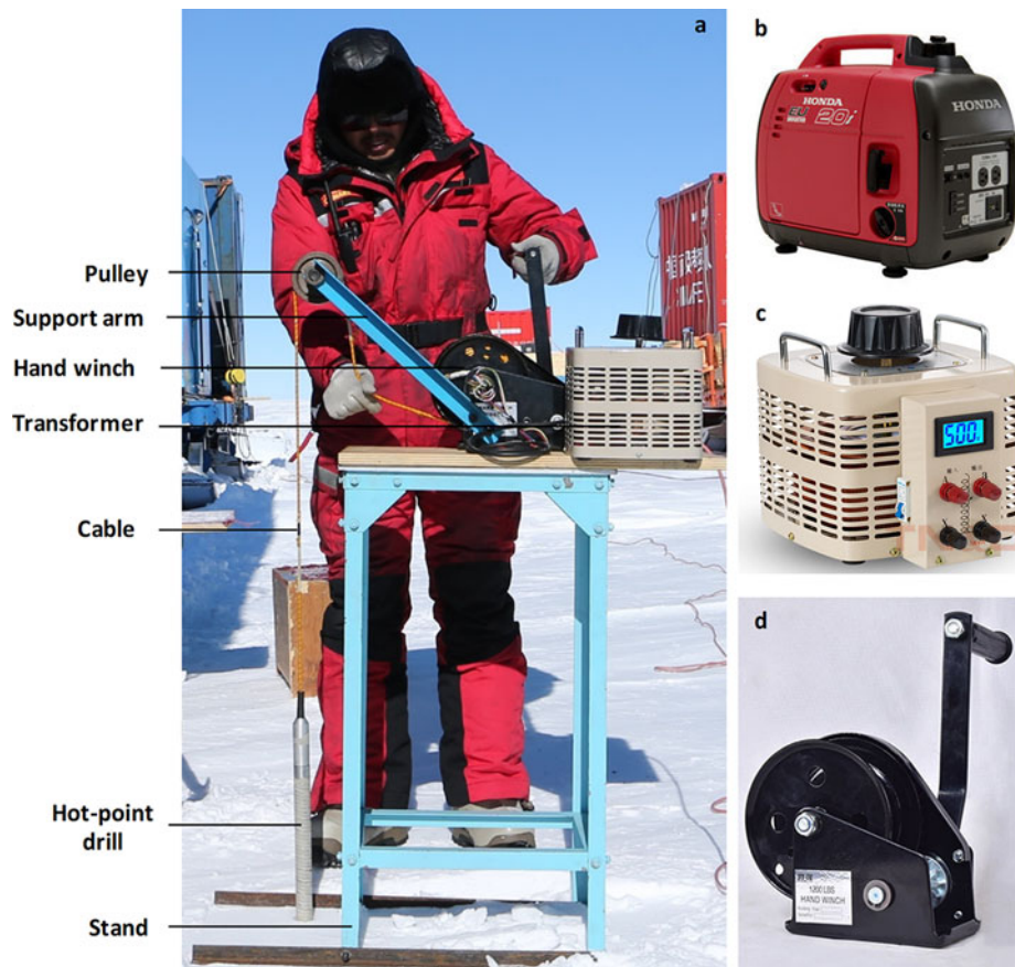
Fig. 1. Overview of (a) shallow hot-point drill system; (b) gasoline generator; (c) transformer; (d) hand winch.
