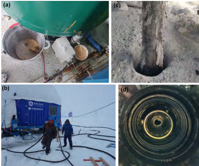
Figure 9. Test phenomena: (a) cyclone dust collector worked well in domestic test; (b) condensed water could not be discharged from the receiver; (c) burying the rubber hose into snow to cool compressed air; (d) condensed water refrozen on the outer surface drill pipe; (e) ice plug formed in drill pipe.
