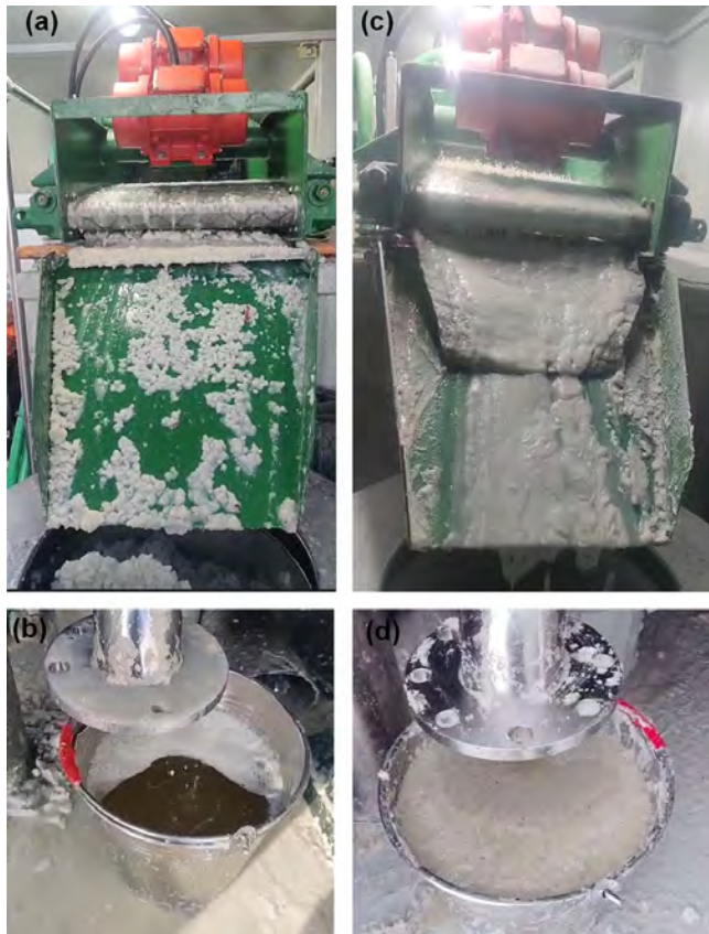
Figure 11. Performance of vibration sieve and vertical centrifuge: (a) small ball of ice chips formed on 100 meshes screen; (b) cleaned drilling fluid when using 100 meshes screen; (c) clogging of 120 meshes screen by ice chips and clay additives; (d) ice chips remaining in the drilling liquid when using 120 meshes screen.
