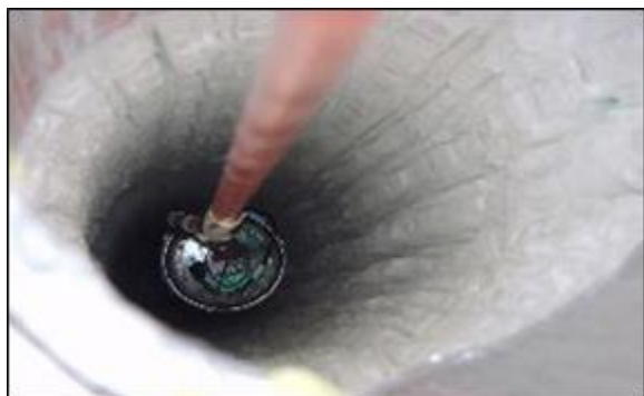
A Digital Optical Module (DOM) is lowered into a hole in the ice at Amundsen-Scott South Pole Station for the IceCube project. IceCube detects neutrinos from distant astrophysical sources. Photo credit: Ethan Dicks, National Science Foundation.
