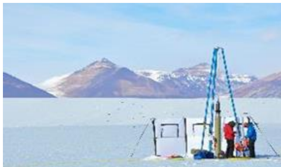
Caption: A large-volume ice core drilled on the Taylor Glacier ablation zone, Antarctica. Bubbles in the ice at the site contain evidence of ancient atmospheric composition. The Blue Ice Drill is an easily-transportable drill capable of retrieving quality firn cores of approximately 9.5 inches in diameter as well as quality solid ice cores of the same diameter up to 70 meters below the firn-ice transition. Photo credit: Jeff Severinghaus .
