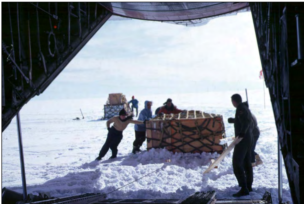
Figure 22. Loading ski-equipped C-130 aircraft with ice cores recovered at Camp Milcent, 1973. Later the cores were temporarily stored in freezers at the Sondrestrom Air Force Base, at the edge of the ice sheet, until the end of the season, when consolidated shipments were made to respective laboratories.
