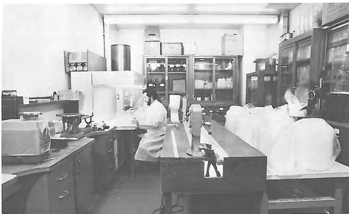
Figure 2. Cold room 160 at USA CRREL used for ice-core processing and study. Temperature of laboratory is -10 \pm 2^{\circ}\text{C} .
