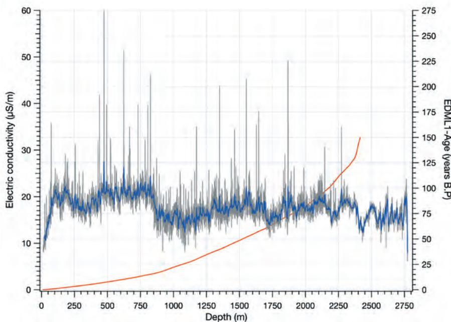
**Fig. 23:** Profile of the electric conductivity of the EDML ice core as measured by DEP in the science trench at Kohnen Station. Shown are temperature corrected ( $-20^{\circ}\text{C}$ ) values. Breaks were not removed. The data are sampled to 0.5-m intervals (grey). The smoothed curve (blue) shows moving averages over 10 m.
