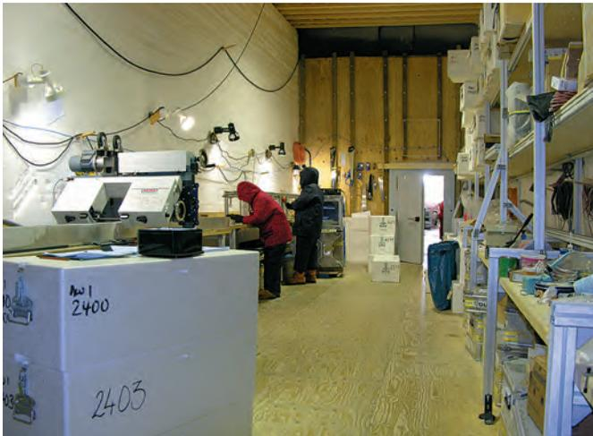
**Fig. 17:** View into the science trench. The band saw on the left side was used to cut the core in 1-m-pieces, which thereafter were measured by DEP. The person in the red clothing is wrapping the core piece for DEP, while the other is observing the measurement. The white PP-foam boxes are used for storage and transportation of the 1-m-pieces, six of them are fitting in one box. (Photo H. Oerter, 23.12.2005).
