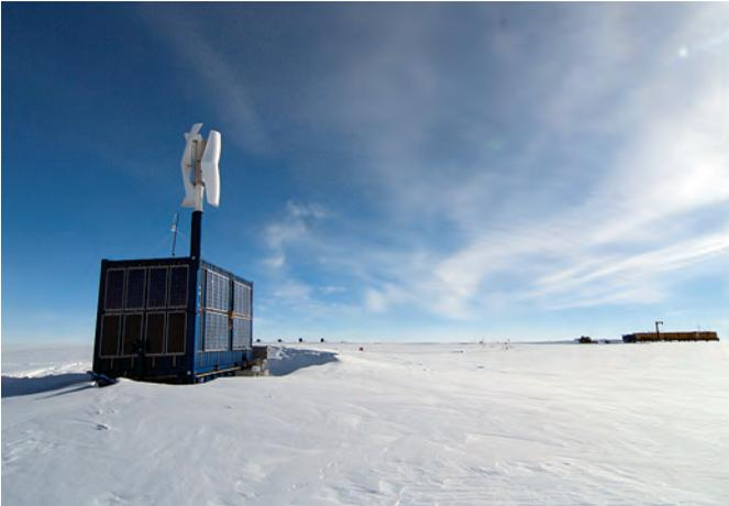
**Fig. 29:** Container with the automatic aerosol sampler inside at Kohnen Station (background right). The air intake is on the roof. Solar panels on the outer walls and the wind generator provide the needed electrical power for year-round charging of the batteries. The container had not been moved during the past two years. (Photo H. Oerter 11.01.2008).
