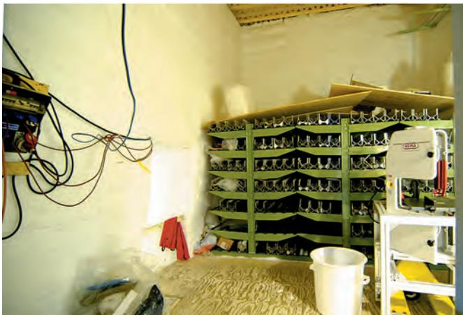
**Fig. 18:** View into the core buffer after drilling operation was finished. The shelf with the core troughs was used for temporary core storage, especially when drilling the so-called brittle zone to allow the cores to get adjusted to the temperature and air pressure in the science trench. On the left, the entrance to the ice cave in the investigation of physical properties is visible. (Photo H. Oerter, 29.01.2008).
