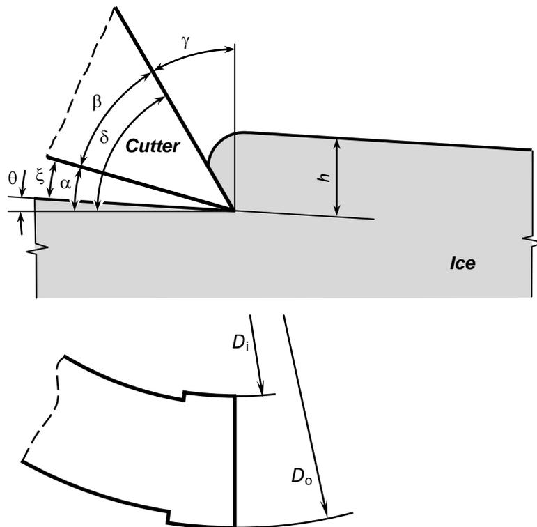
Fig. 15. Schematic of cutter's geometry
