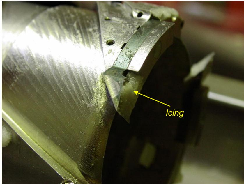
**Fig. 20.** Icing in the warm ice, NGRIP borehole, 4<sup>th</sup> of July 2001
