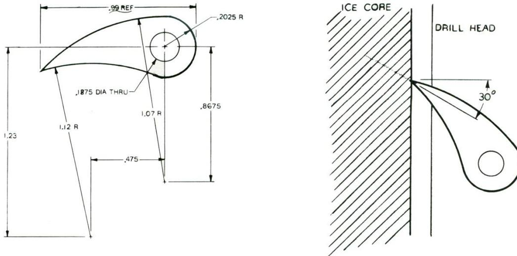
**Fig. 25.** Recommended by Koci (1984) shape of the core catcher (on the left) and core catcher position relative to ice core (on the right)
