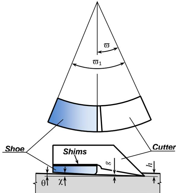
**Fig. 18.** Working scheme of the rear-mounted shoe
