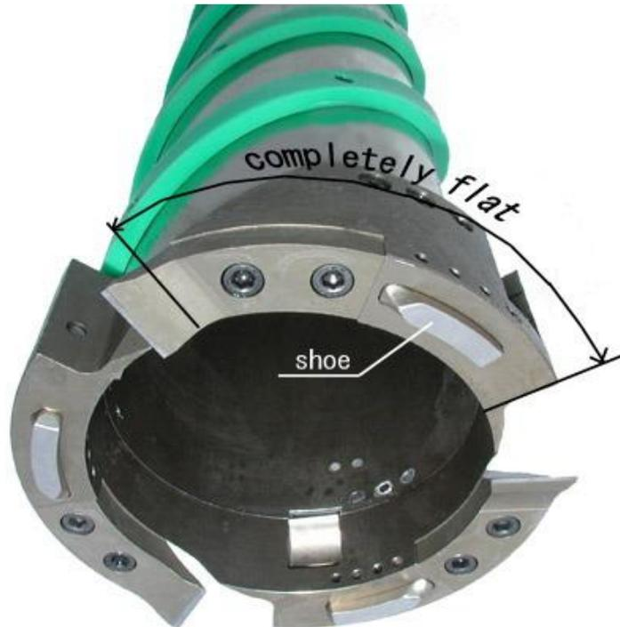
**Fig. 21.** JARE cutters and shoes for drilling in the warm ice
