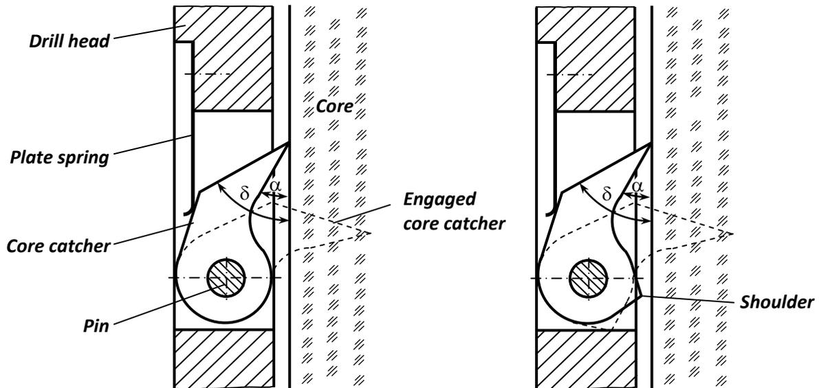
**Fig. 24.** Core catcher of 'dog leg' type: on the left – without shoulder; on the right – with shoulder
