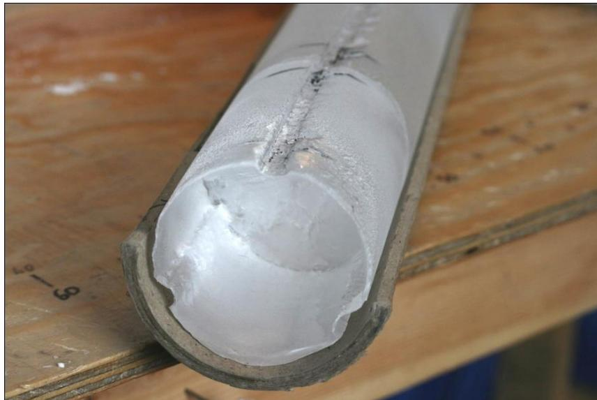
**Fig. 28.** In the warm ice core catchers formed deep long grooves on the surface of the core, Vostok station, Antarctica, January 2007 (Credit: *Alexey Ekaykin*)
