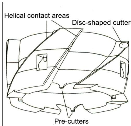
**Fig. 14.** Swiss drill head with pre-cutters and side-wall cutters
