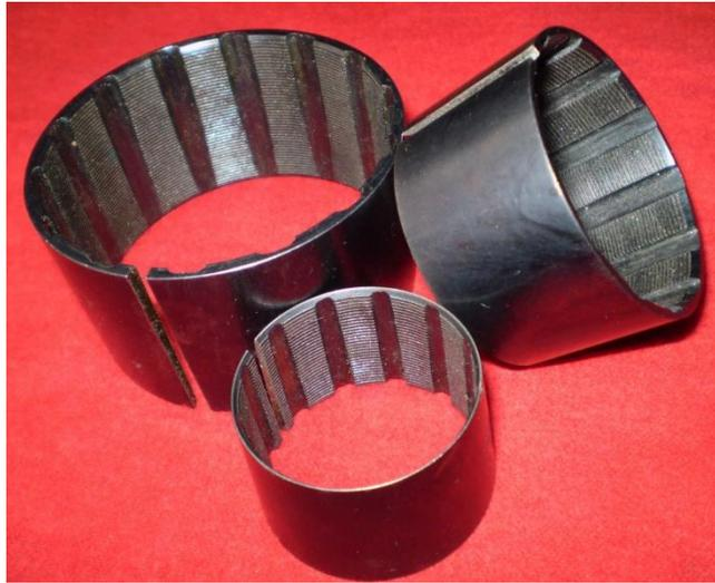
**Fig. 22.** Split-ring core lifters for conventional prospecting drilling
