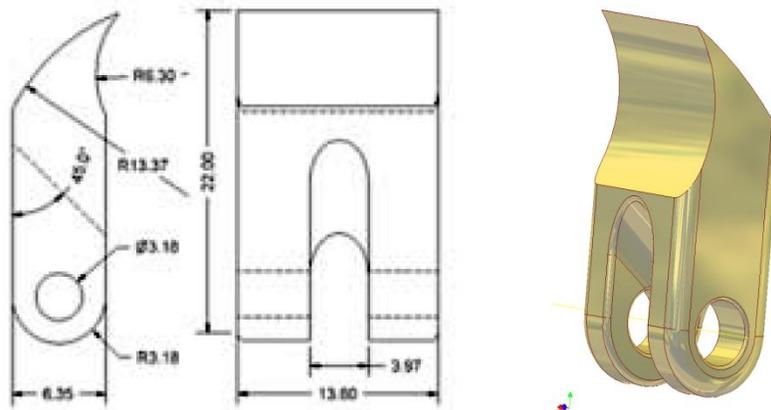
**Fig. 23.** 'Dog leg' type core catchers
