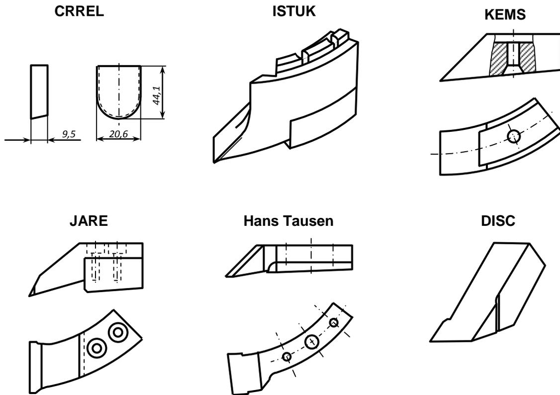
Fig. 9. Shapes and designs of cutters
