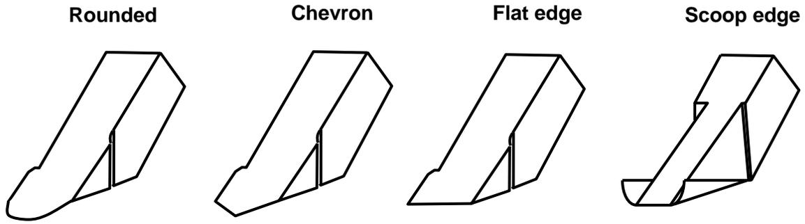
Fig. 8. Tested shapes of the cutter's edge
