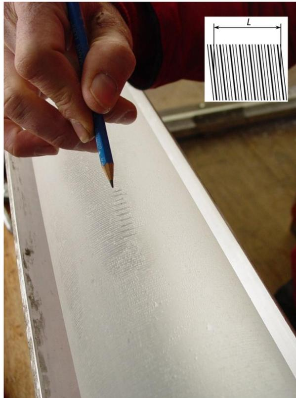
**Fig. 7.** Estimation of the pitch and cutting depth
