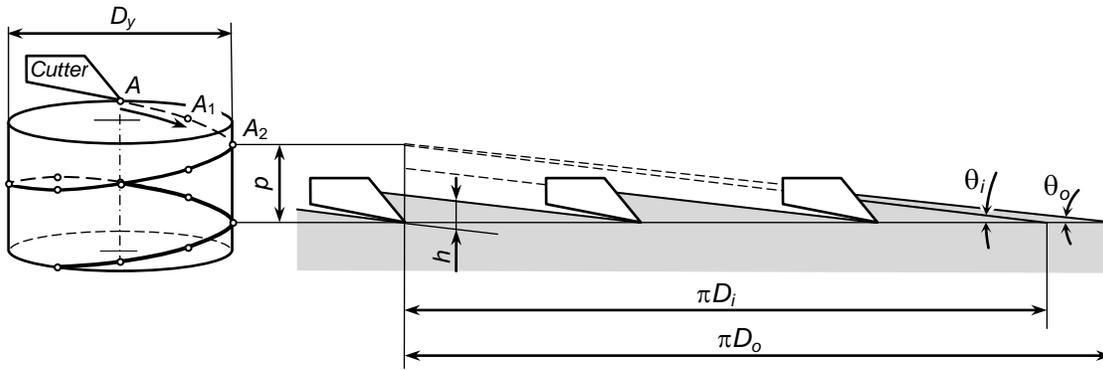
**Fig. 6.** Schematic of a three-cutter drill head moving mode
