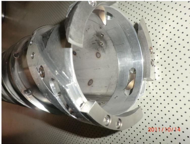
**Fig. 29.** Core catchers for reverse cutting neck on the core surface (hand auger designed by *H.Ruffli*, picture was taken by author in AWI)
