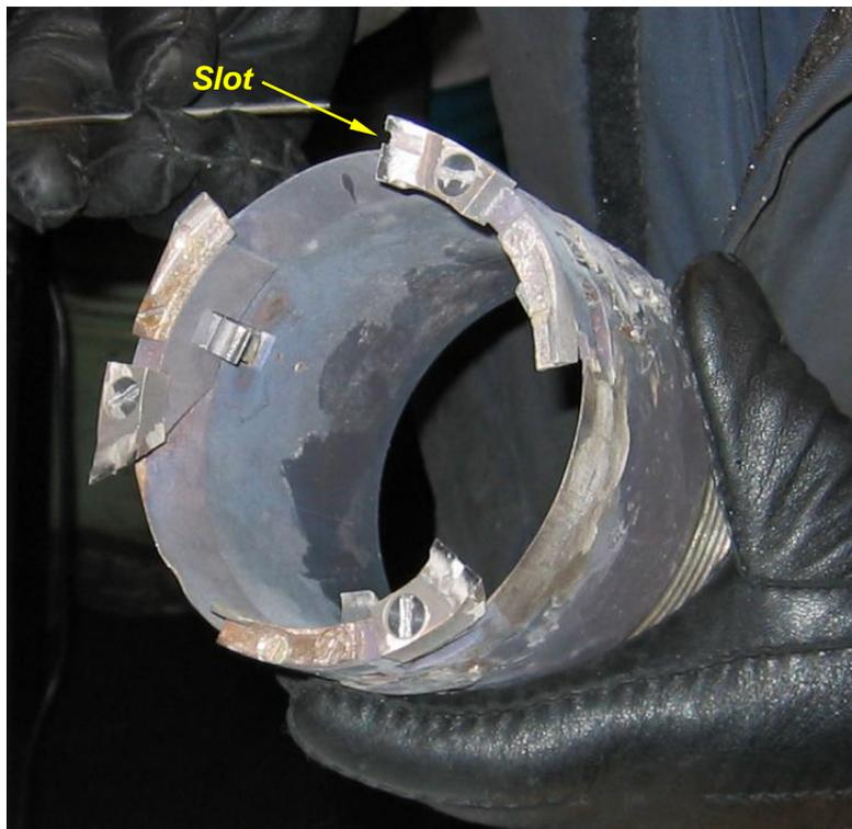
**Fig. 10.** KEMS drill head with special slotted cutters for drilling in the warm ice, Vostok Station, January 2006 (Credit: Alexey Ekaykin)
