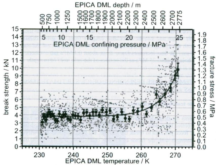
**Fig. 27.** Fracture stress of the core versus temperature estimated in EPICA DML borehole (*Wilhelms et al., 2007*)
