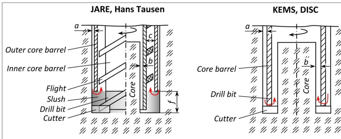
**Fig. 4.** Schematic of the near-bottom circulation
