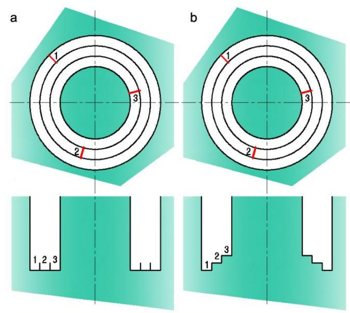
**Fig. 12.** Borehole bottom shaping with staggered cutters (a) and step-staggered cutters (b) (*Zagorodnov et al., 2009*)
