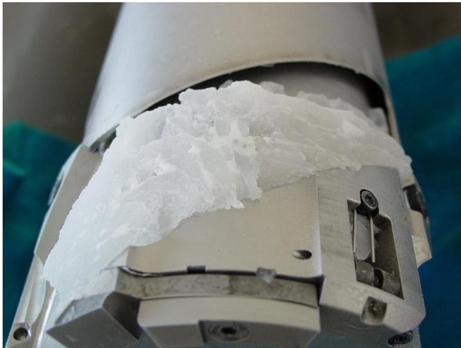
**Fig. 3.** Hans Tausen drill head with the buildup of ice that occurs in the warm ice, Dome C, Antarctica (Credit: *Laurent Augustin, EPICA*)
