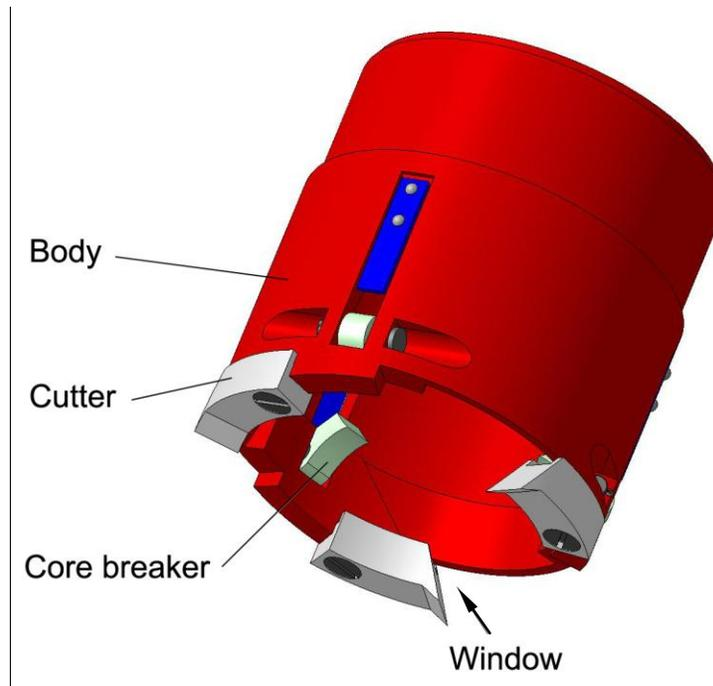
Fig. 5. KEMS drill head
