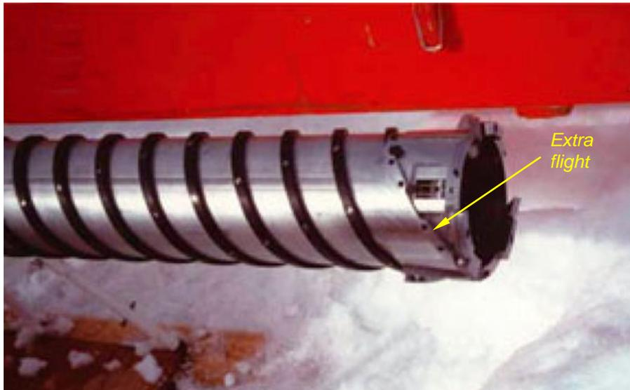
**Fig. 2.** Extra flights on the Hans Tausen drill head extending to the hole wall produced immediate packing (*Johnsen et al., 2007*)
