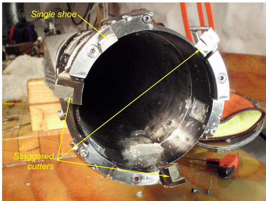
**Fig. 13.** Staggered cutters mounted on the Hans Tausen drill-head, NEEM, July 2010 (Credit: *Steffen Hansen*)
