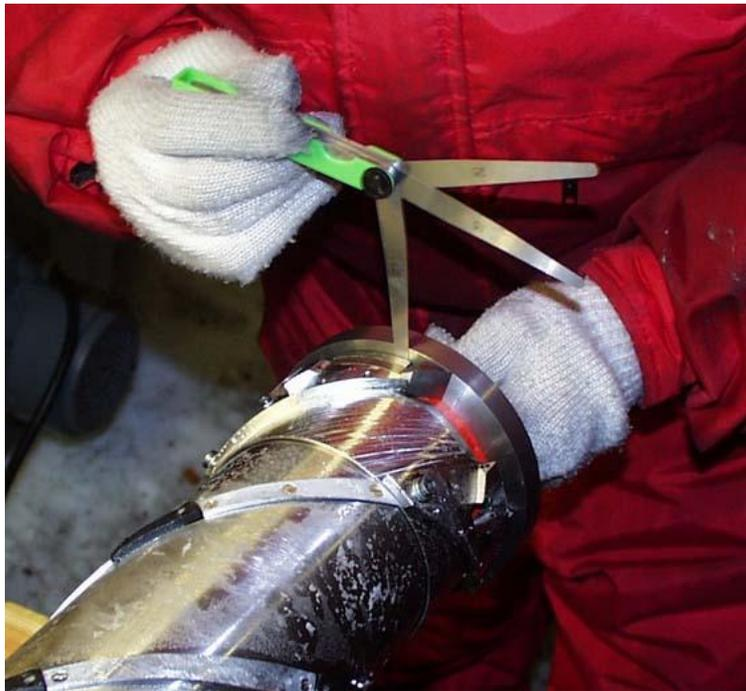
**Fig. 19.** Measurement of the shoe clearance, Hans Tausen drill head
