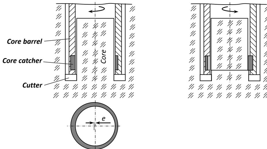
**Fig. 30.** Eccentric core catcher working at reverse rotation of the core barrel
