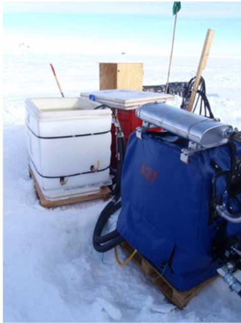
Figure 10: ASIG Engine Covers: Cover is sealed to drip pan on base with Dual-Lock industrial Velcro. Outlet flaps, open during operation, are sealed for storage.
