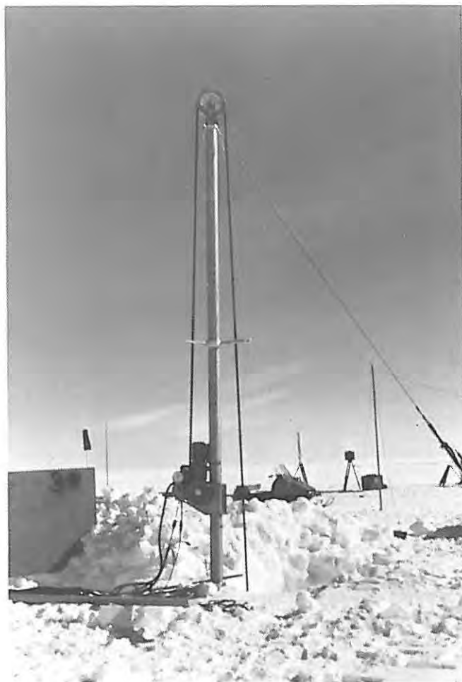
Figure 9. Drill unit assembled at Summit Station, Greenland.
