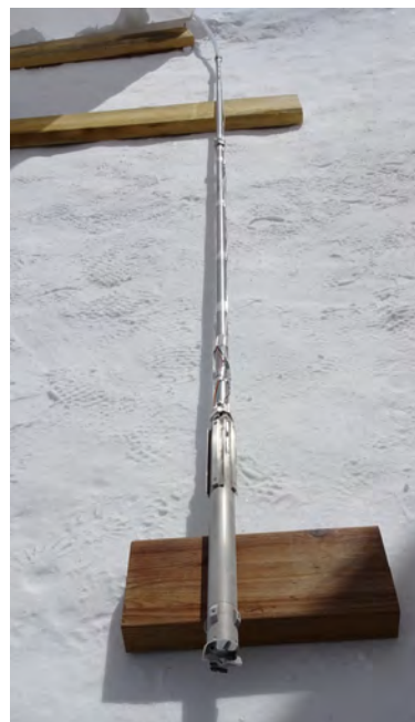
Figure 3. A 40 mm firn drill on a vacuum line for lifting ice cuttings. All pieces were manufactured in the workshop of the Physics Institute, University of Bern.
