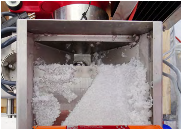
Figure 9. Top view of fluid–chip separation on a slotted wedge wire screen. The slurry is moving upwards on the vibrating screen and falls into the screw press below.
