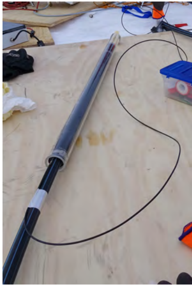
Figure 4. Packer inserted into a Plexiglas tube to test inflation. The inner diameter of the tube is identical to the borehole diameter.
