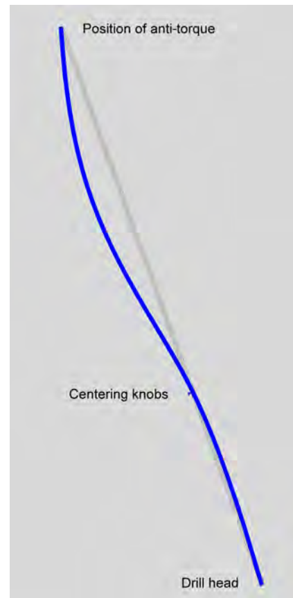
Figure 12. Bending of drill by gravity (exaggerated). Finite-element simulation with actual material properties and tests with the drill itself led to an optimal position of the centering knobs at about one-third from the lower end.
