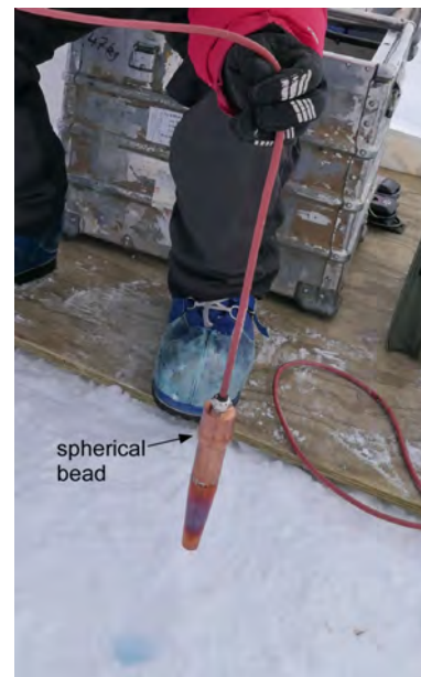
Figure 2. Heated copper “plumb bob” for melting and glazing the first 6 m of the firn hole.
