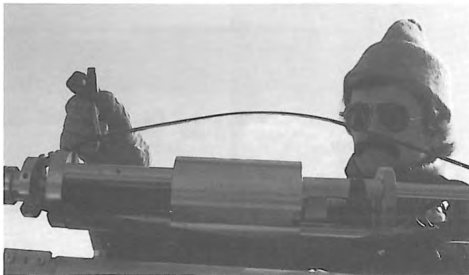
Fig. A27. Antitorque skates in assembly.
