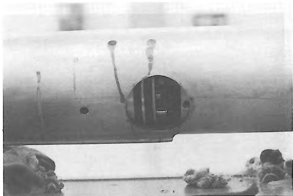
Fig. A14. Piston seals may be damaged during disassembly when they pass the leading edge of this opening.
