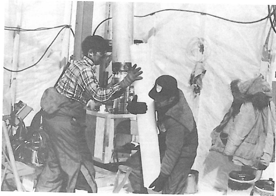
Fig. B-7. Core removal, sometimes a two-man job.
