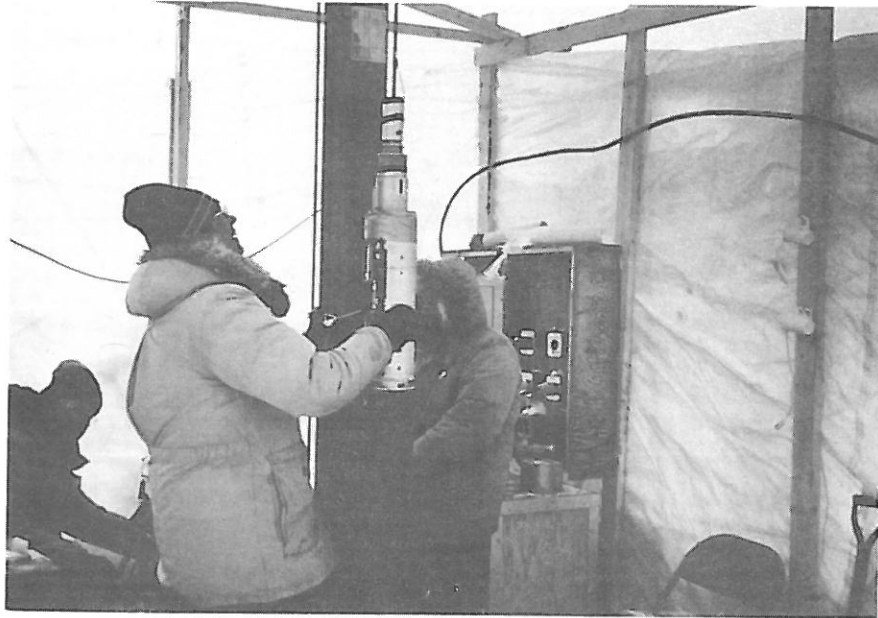
Fig. B-3. Alcohol being drawn through the vacuum pump to clear moisture and ice from lines.
