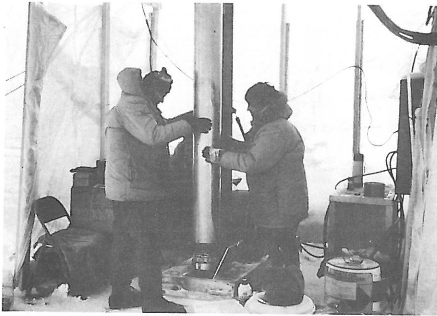
Fig. B-5. Once the operational checks have been made the drill is ready to be lowered downhole again.
