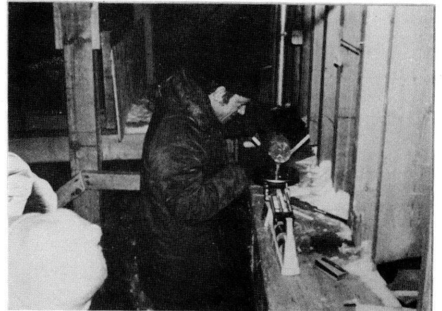
b. Smoothing sample ends in a steel V-block.
