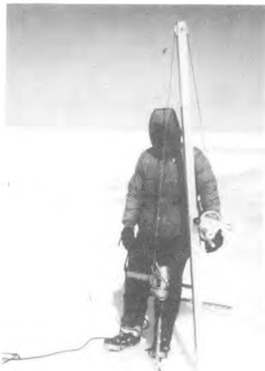
Figure 18. Simple gin-pole for lifting long sections of auger (can also be used to lift small ice blocks).
