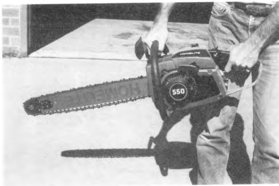
Figure 14. Standard gasoline chain saw with 20-in. bar.
