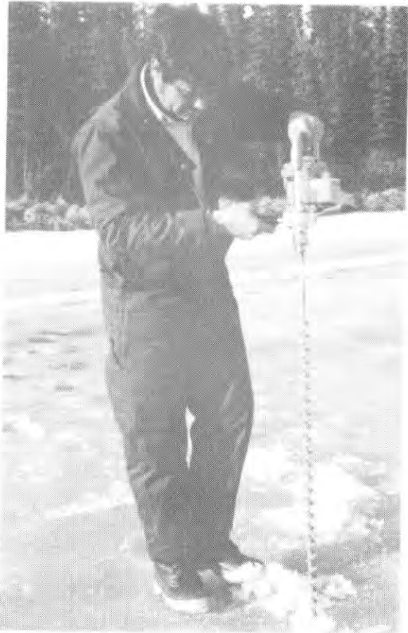
Figure A3. Very small gasoline drive unit on small-diameter ice auger.
