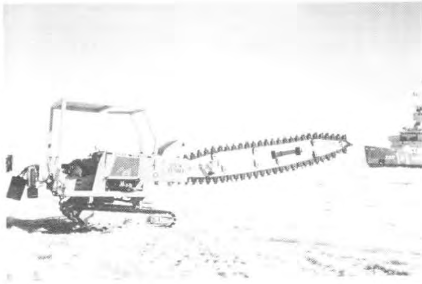
Figure 13. Ice saw developed by NCEL.
