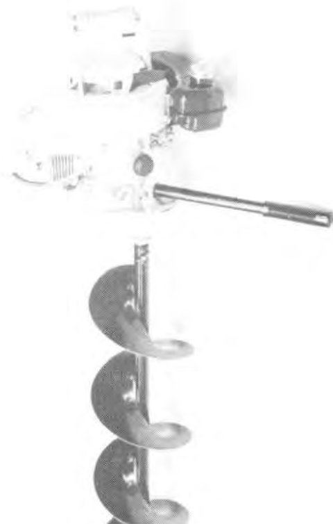
Figure A9. Three-horsepower gasoline drive unit on 9-in.-diam auger. The simple gearing gives left-hand rotation. The simple straight handle for torque reaction is considered safer than looped butterfly handles, which have been known to break the operator's arm.
