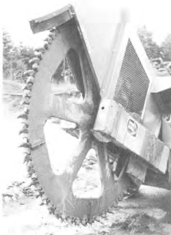
Figure 17. Ditch-Witch disc saw. These machines have been used for cutting ice near Prudhoe Bay.
