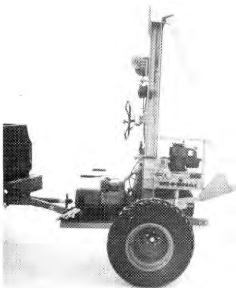
Figure A12. Small drill rig for making large diameter holes in thick ice. The mast extension is folded down, and a small generator is stowed on the operator's platform.
