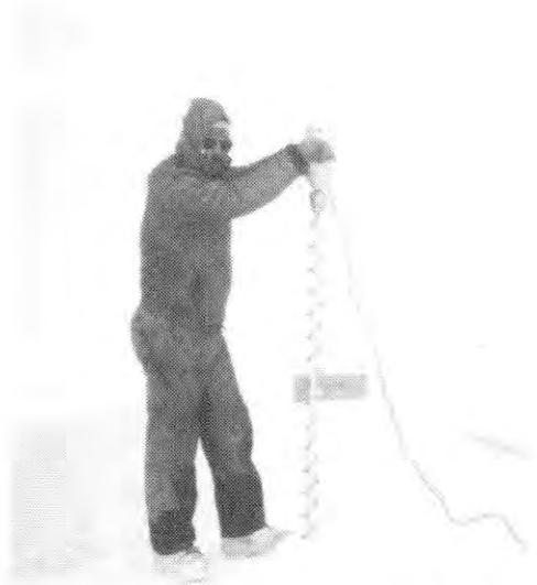
Figure A1. Electric drive unit on 3 1/4-in.-diam ice drill.
