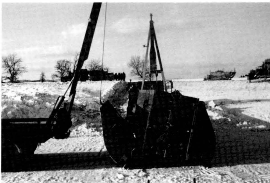
d. The second bow ponton was closed by lifting it with a second transporter.
