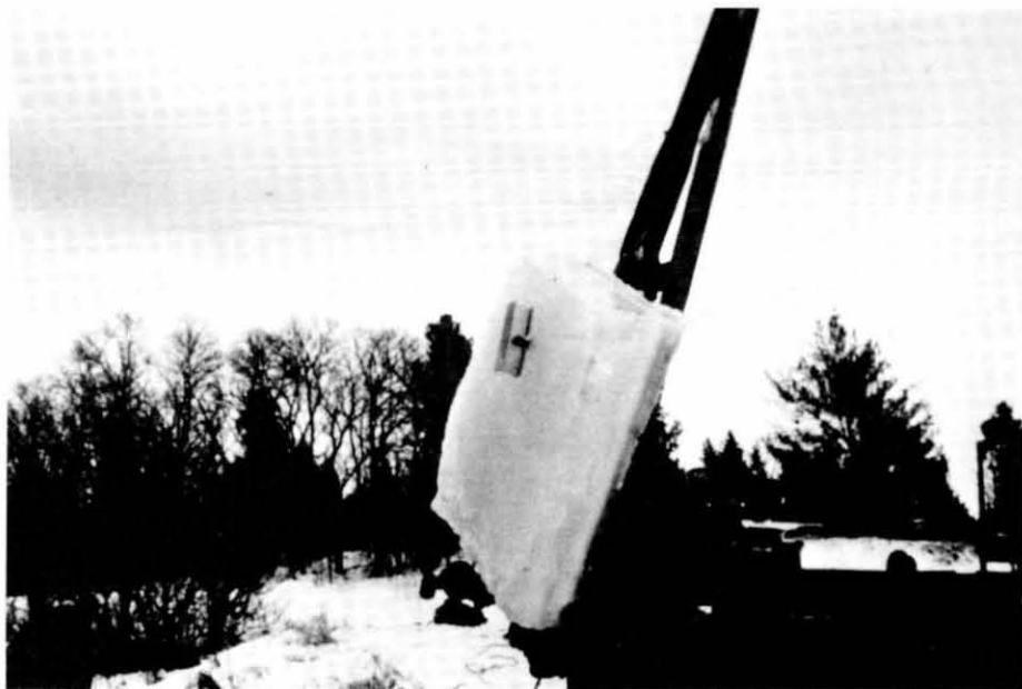
Figure 7. Ice block lifted by a transporter and being laid against the boom as it is lowered to the cradle.
