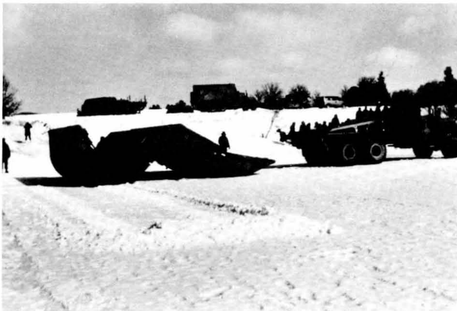
a. The cable from the transporter slowly pulled the bow ponton to start the bay unfolding.
