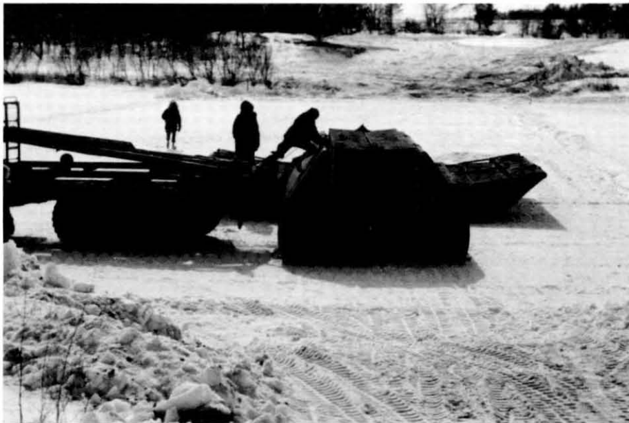
b. A transporter was again needed to start the bay unfolding.
