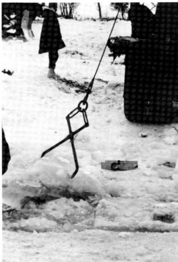
Figure 8. Lifting ice blocks with timber tongs. The edge of the ice shown here has already spalled off once from a previous attempt to lift it using the timber tongs; the points of the tongs are only gripping at the edges of the ice.
