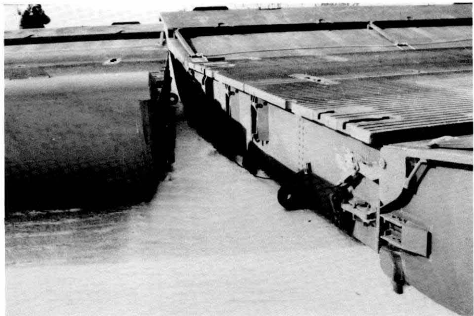
Figure 13 (cont'd). Opening a second bridge bay.
