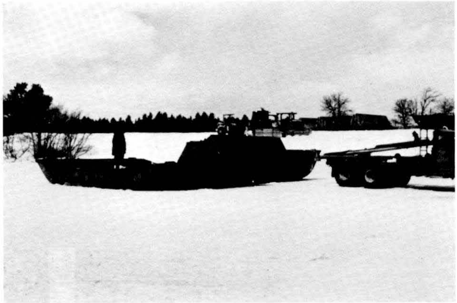
c. The bay unfolding as the transporter is pulling the bow ponton.
