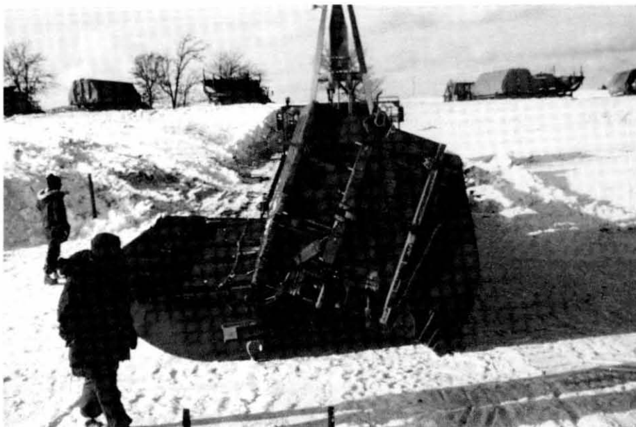
c. One bow ponton was coaxed closed by cycling the bay up and down.
