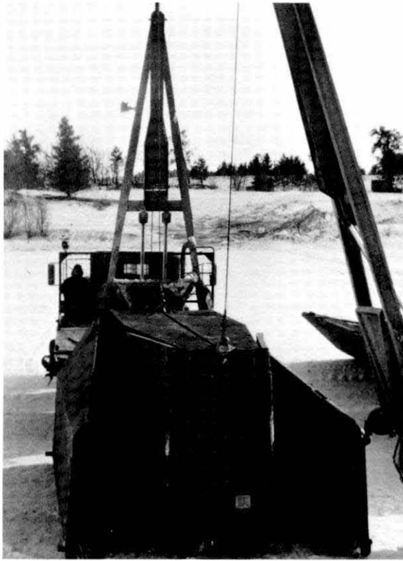
a. The ramp bay with both transporters attached. Lifting up both ends of the bay allowed the bow pontons to rotate closed.
