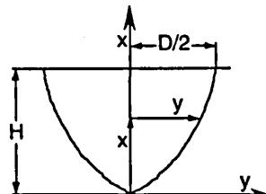
Figure 7. Paraboloid geometry.
