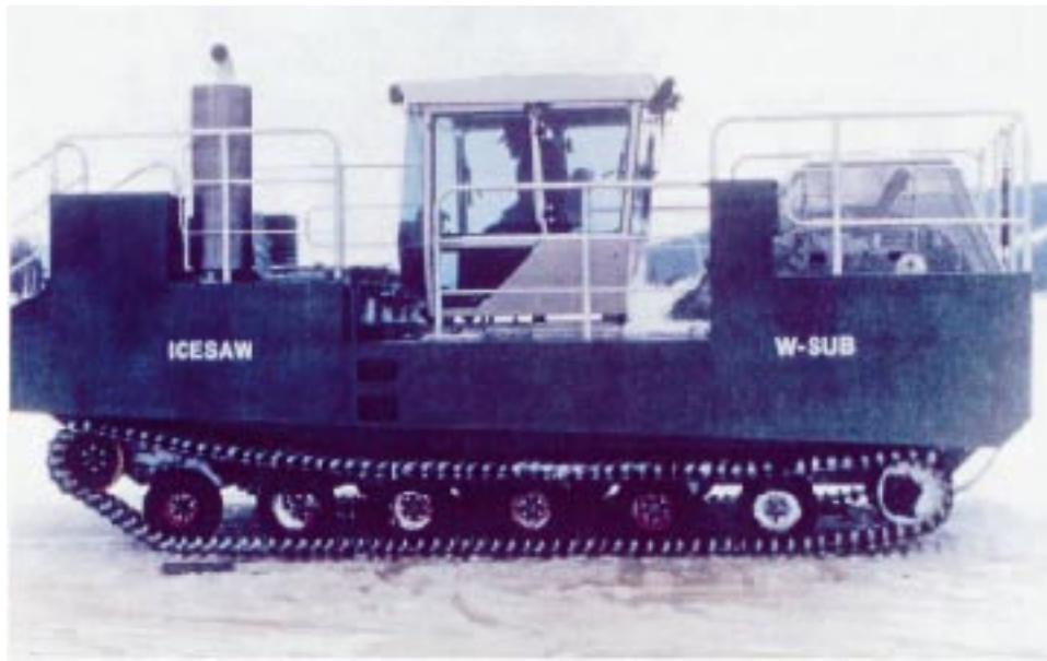
Figure 3. ICESAW used for cutting river ice (photo courtesy of Mobimar, Ltd.).
