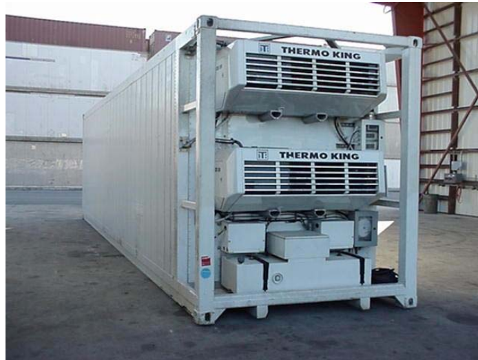
Figure G1. Nose mount Reefer (dual coolers with integral gensets)
