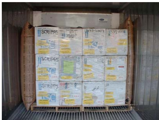
Figure E13. Existing cardboard ISC4 stacked 3-high inside reefer.
