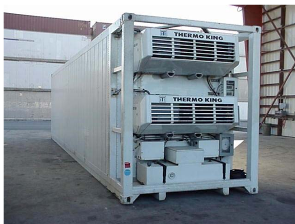
Figure 2. Nose mount reefer (redundant coolers with integral gensets)
