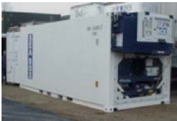
Figure 4. Window-Frame Reefer with single cooling unit (bottom of picture) and clip-on genset (top of picture). Redundant systems not shown.
