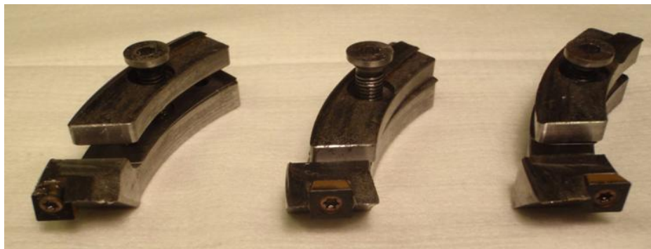
Fig. 40. Step cutters with carbide inserts (Photo: S. Hansen)
