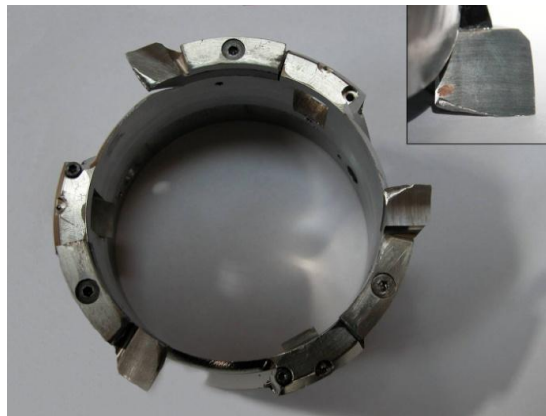
Fig. 35. Damaged cutters while hitting bedrock, NorthGRIP, 2004 ( NGRIP ice core drilling project, www.gfy.ku.dk )
