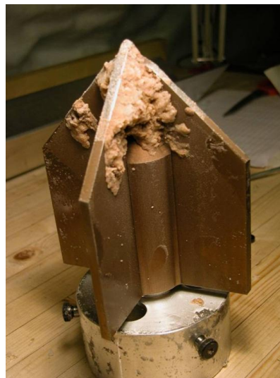
Fig. 36. Conical scraper with icy-muddy slush from the bedrock of NorthGRIP hole, 2004 ( NGRIP ice core drilling project, www.gfy.ku.dk )
