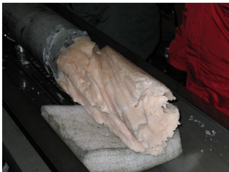
Fig. 34. Refrozen subglacial water hanging underneath Hans Tausen drill, NorthGRIP, 2003 (NGRIP ice core drilling project, www.gfy.ku.dk )
