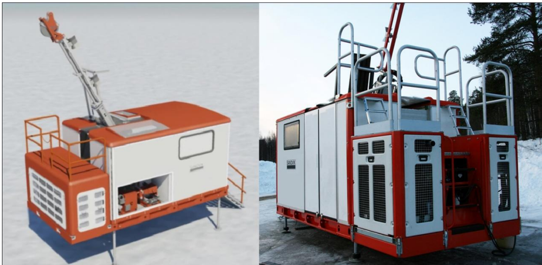
Fig. 14. Sandvik Drill Shack for intermediate drilling in Arctic and Antarctica (at the left) redesigned from commercial version for temperate climate (at the right) ( www.sandvik.com )
