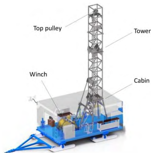
Figure 1. Structure of the movable polar drilling shelter.
