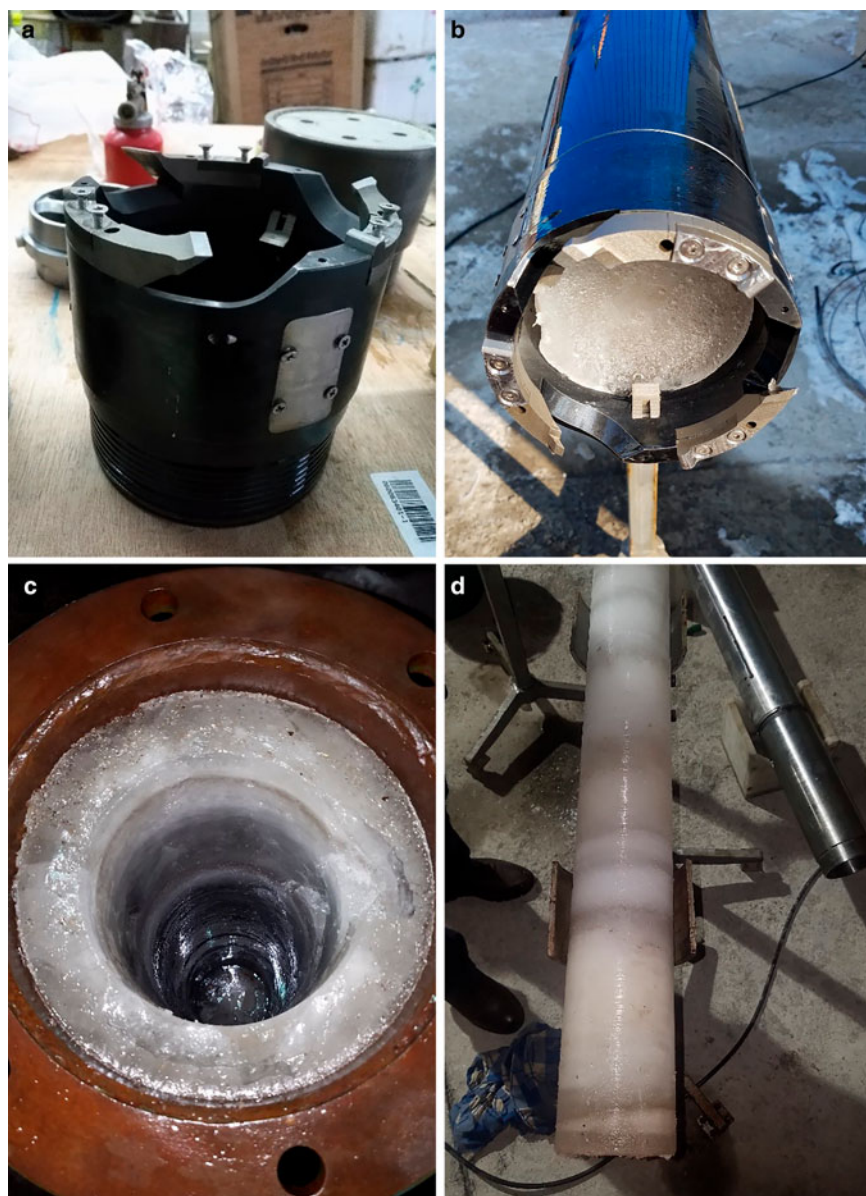
Fig. 4. Ice-drilling tests of the shortened version of the IBED at the outdoor testing stand: (a) ice-drill head; (b) core barrel with the ice core; (c) borehole drilled in an ice sample; (d) recovered ice core.
