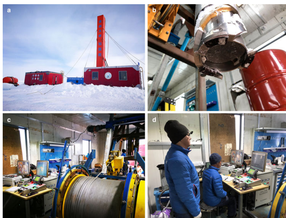
Fig. 11. Drilling operations at the JLU drilling site in the vicinity of Zhongshan Station, East Antarctica: (a) drilling camp; (b) auger version of the IBED with the ice core; (c) drilling winch and control desk; (d) drilling process monitoring.
