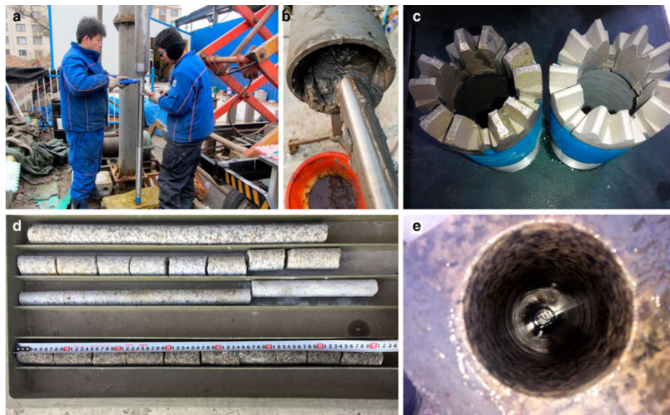
Fig. 9. Tests of the IBED on granite blocks at the outdoor testing stand: (a) assembling the drill; (b) bedrock chips; (c) worked-out and new toothed impregnated drill bits; (d) recovered bedrock core; (e) bedrock borehole.
