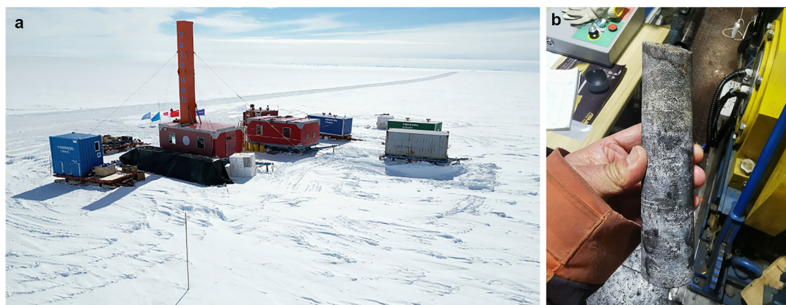
Fig. 2 | Drilling to the bed at the northwestern Princess Elizabeth Land, East Antarctic Ice Sheet. a Bird's eye view of the drilling camp showing the drilling shelter, workshop, living shelters, and auxiliary facilities in northwestern Princess
