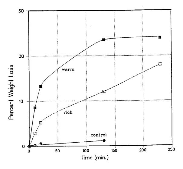
Figure 1. Attack of ice by aqueous alcohol warmer or richer than equilibrium conditions.
