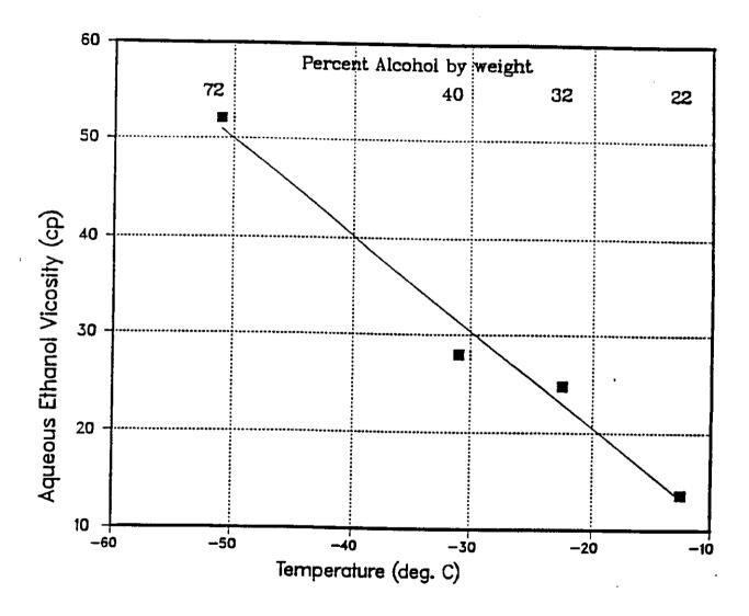
Figure 4. Viscosity of aqueous ethanol solutions at their freezing point. (Percent alcohol content by weight is shown at the top of the figure.)
