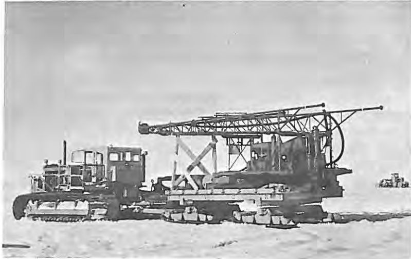
Figure 6. Failing 314 mounted on 10-ton sled prior to installation in trench.
