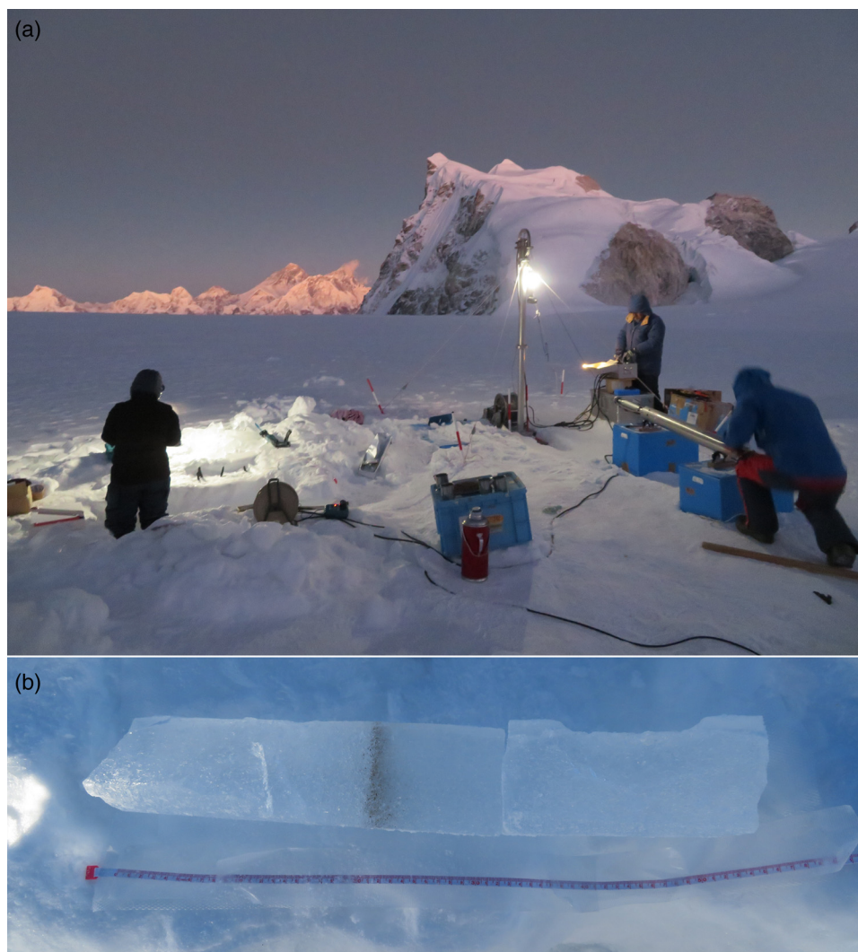
Fig. 2. Photographs of the drill system (a) and in situ ice core processing (b; run no. 82) on the Trambau Glacier during the 2019 drilling expedition.
