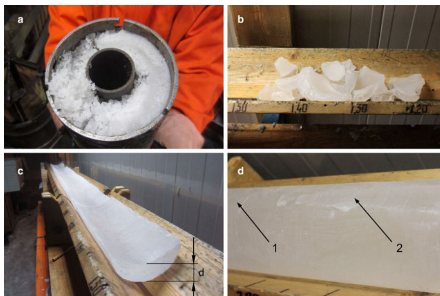
Fig. 6. (a) Run 1: chips in the chip chamber after milling a shallow ledge in the 5G-1 hole at a depth of 3277 m. (b) Run 4: fragments of crescent ice core, recovered from 3280 m. (c) Run 6: intact crescent ice core, 3285 m: d – thickness of the core cross-section. (d) Run 16: full diameter core, 3291 m: 1 – surface of the 5G-5 ice core; 2 – wall of the 5G-1 hole.
