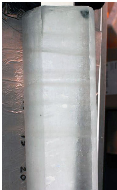
Fig. 7. Ash layers in the 5G-5 ice core used to anchor this new core on the 5G-1 ice core logging depth taken as reference.
