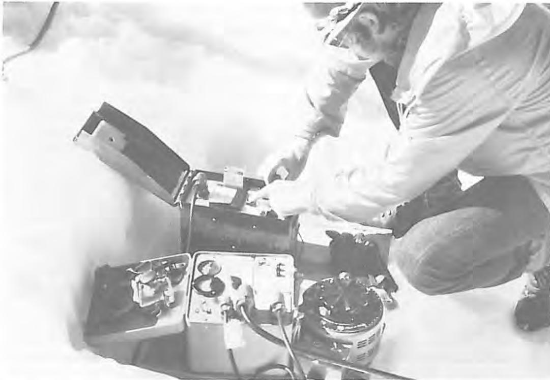
Figure 3. Coring drill controls. Operator is reading the inclinometer prior to core breakoff and retrieval. Drill power controls in the foreground.
