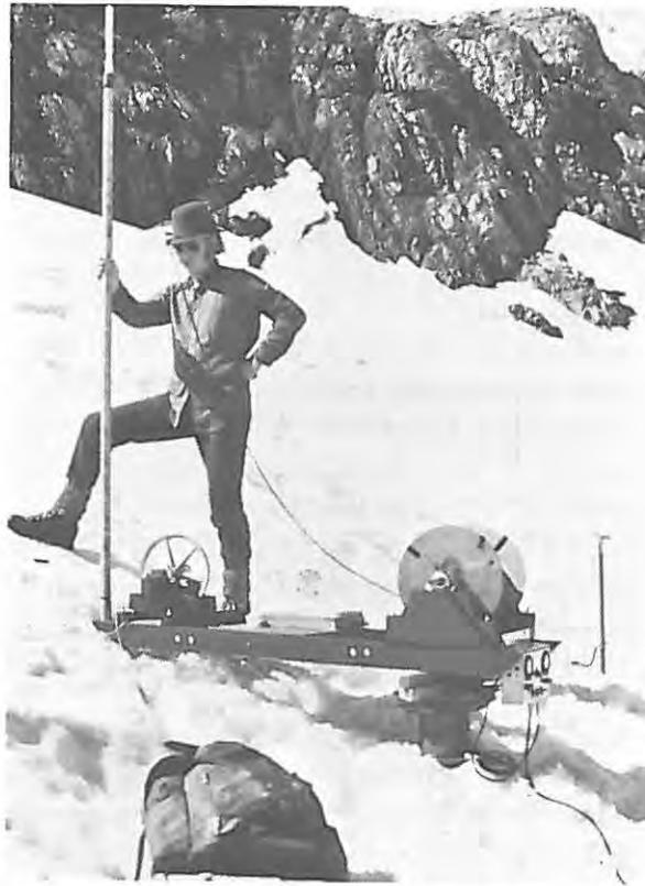
Figure 7. Solid-nose drill platform. Operator holds the drill stem; cable has been lifted off the meter wheel sheave. Cable drum and power control box on the right.
