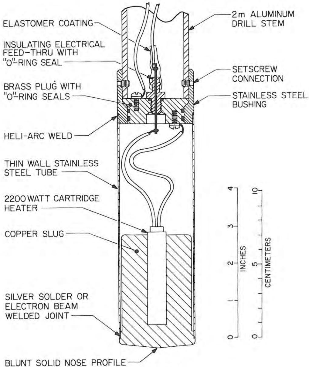
Figure 5. Cross section of the solid-nose hot-point drill.
