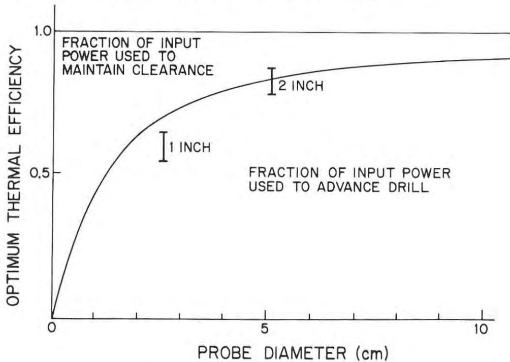
Figure 8. Optimum thermal efficiency for solid-nose hot-point drills operating in wet temperate ice. Clearance diameter is 5 mm between probe and hole. Bars show range of observed values.
