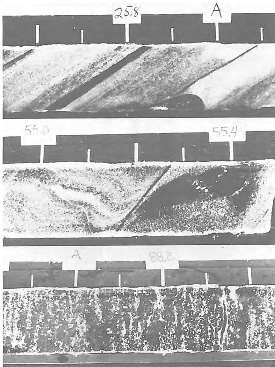
Figure 4. Samples of a continuous vertical core taken near the base of the icefall, Blue Glacier, Washington, 1971. Numbers indicate depth from the surface in meters; scale divisions are decimeters.
