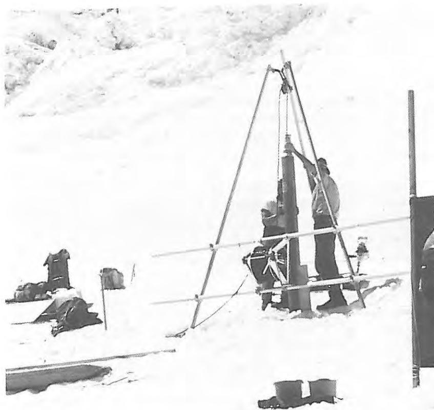
Figure 1. The thermal coring drill. Winch installation on the near side of the supporting tripod.
