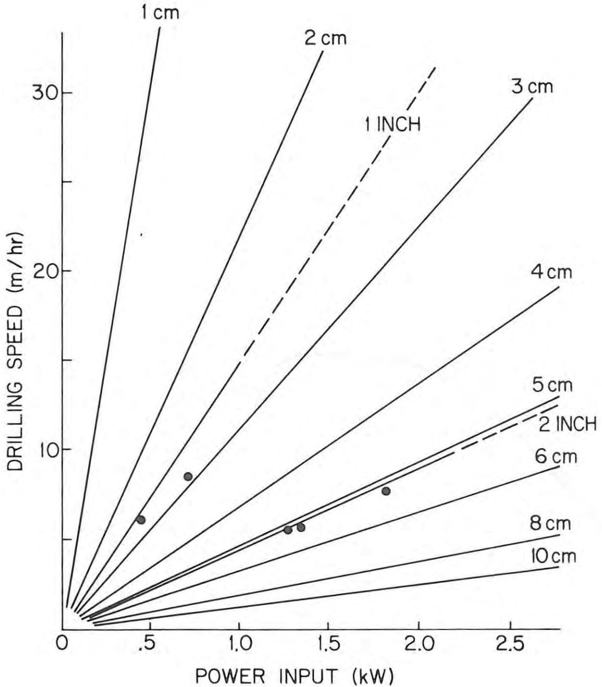
Figure 9. Drilling speed and power input for solid-nose hot-points operating at the optimum thermal efficiency shown in Fig. 8. Observed values for the 1-in. and 2-in. drills are shown as dots; dashed extensions are for power input above the cartridge rating.
