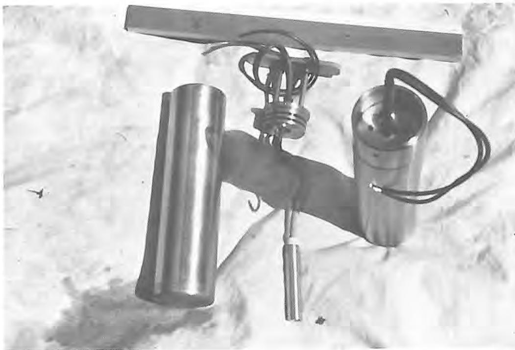
Figure 6. Solid-nose hot-point assembled, and with plug and heater assembly removed with small pulling tool. Scale in inches.
