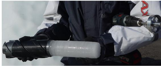
**Fig. 5.** After drilling and removing the core, the shaft is detached from the drill and the sample is extracted. Here, the ice sample is displayed, but normally it would be placed directly into a sterile plastic bag and into a freezer for later analysis.
