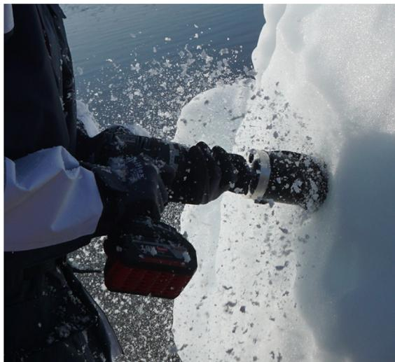
**Fig. 3.** Sample acquisition underway on a grounded bergy bit in western Greenland. The sleeve efficiently removes ice cuttings. Note that the drill could be placed inside a plastic bag in warm weather if ice cuttings were to land and melt on the drill.
