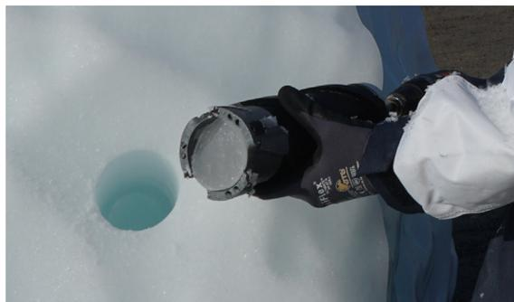
**Fig. 4.** A detached core held in place by the core dogs with a clean borehole visible in the background.
