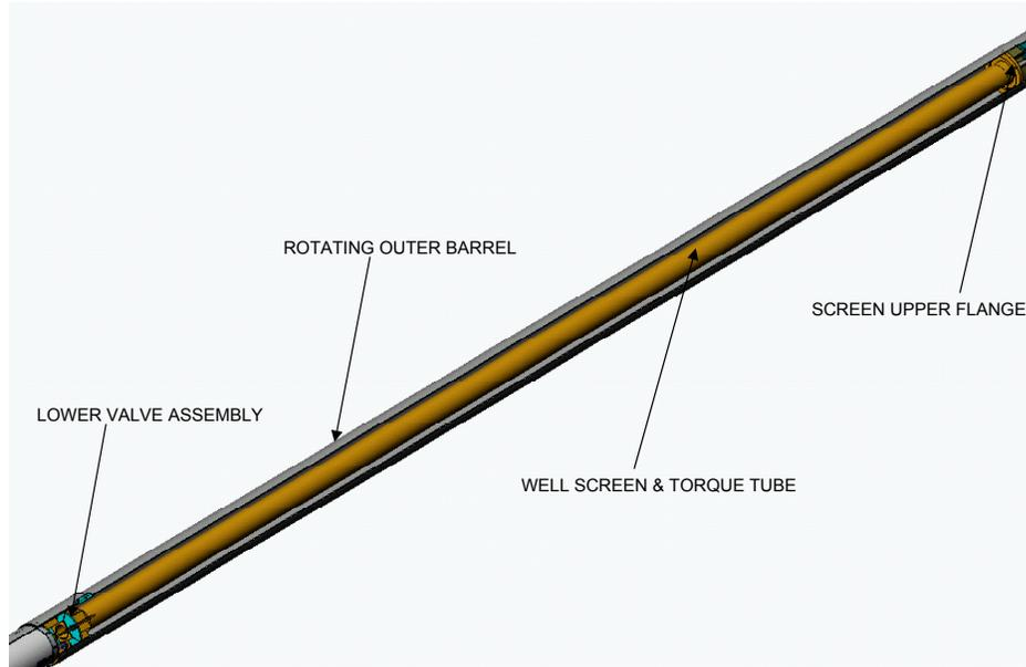
**Figure 11 Well Screen Filter Assembly**
