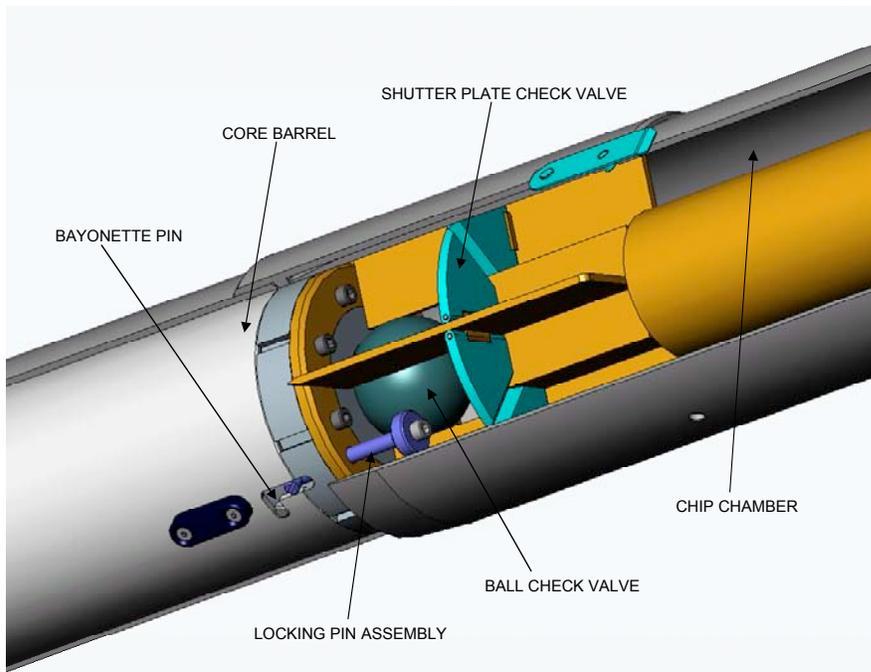
**Figure 12 Lower Valve Assembly**
