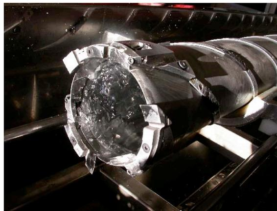
**Figure 5: Coring Head with Ice Core**
