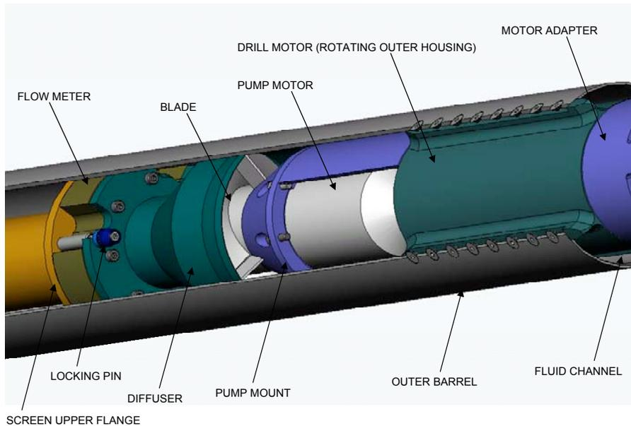
**Figure 10 Motor and Pump**
