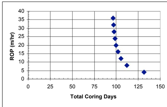
Figure A-6: Rate of Penetration Effect on Total Coring Days
