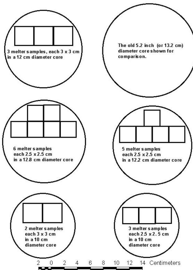
**Figure 19: Ice Core Cutting Plan**
