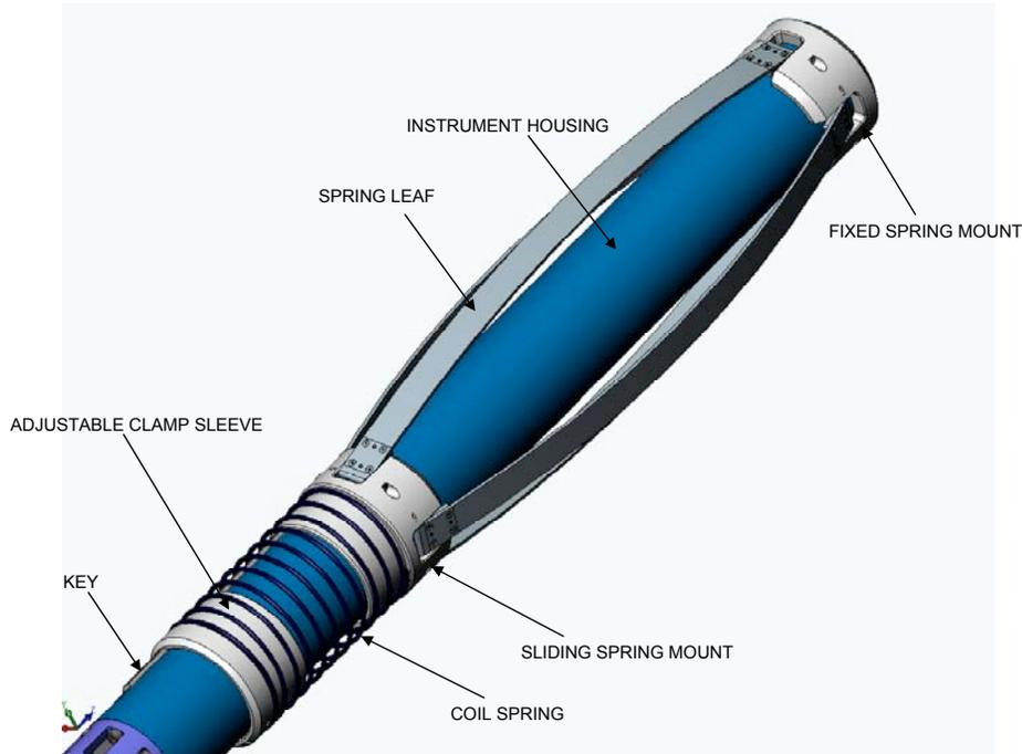
**Figure 8 Instrument section and Anti-torque assembly8**
