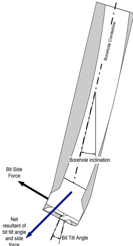
**Figure 22: Bit Tilt and Side Force**
