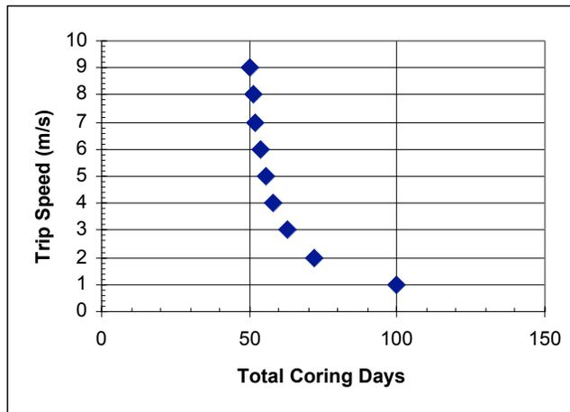
**Figure A-3: Trip Speed Effect on Total Coring Days**
