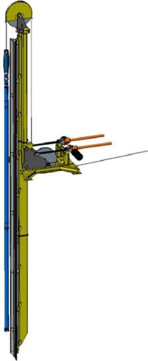
Figure 17 Sonde and tilting tower - vertical
