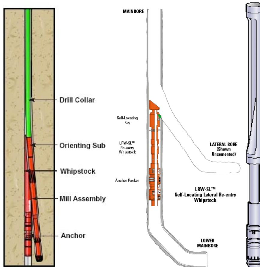
Figure 24: Whipstocking Process (from RMOTC and Halliburton web sites)
