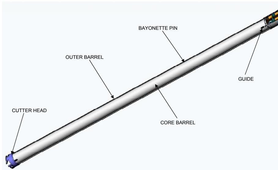
**Figure 14 Core barrel assembly**
