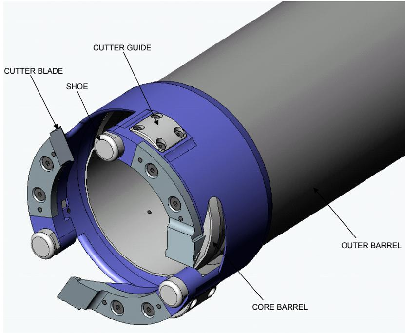
**Figure 16 Disk cutter head**
