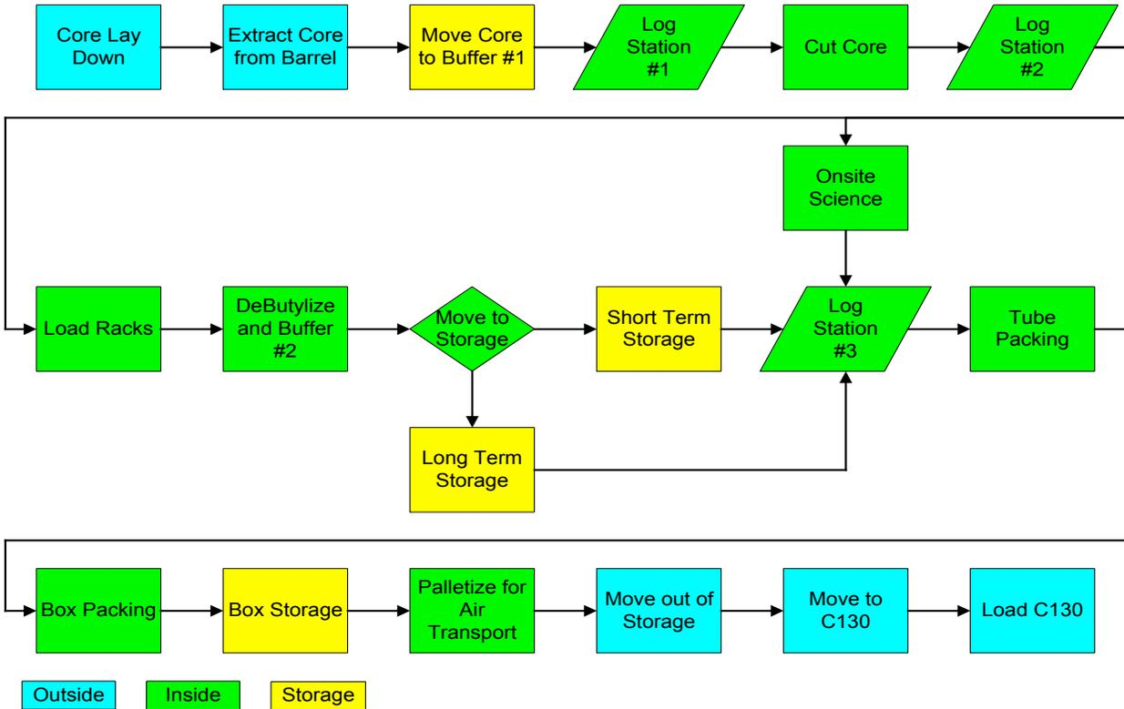
Figure 21: Field Ice Core Handling Train
