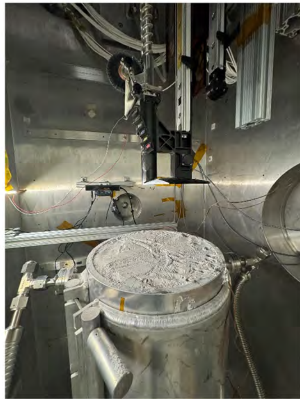
Figure 12. Environmental test chamber used to simulate a lunar environment for TRIDENT EU testing. The bin is approximately 30 cm in diameter.
