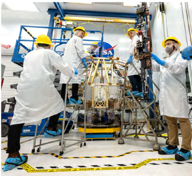
Figure 10. Moments before integrating the VIPER TRIDENT FU into the chassis of VIPER at Johnson Space Center in Houston. Courtesy NASA Bill Stafford.
