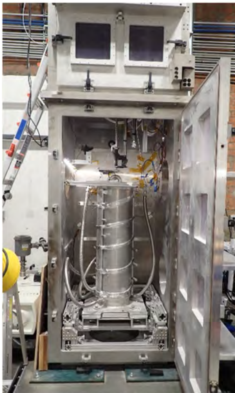
Figure 12. Environmental test chamber used to simulate a lunar environment for TRIDENT EU testing. The bin is approximately 30 cm in diameter.
