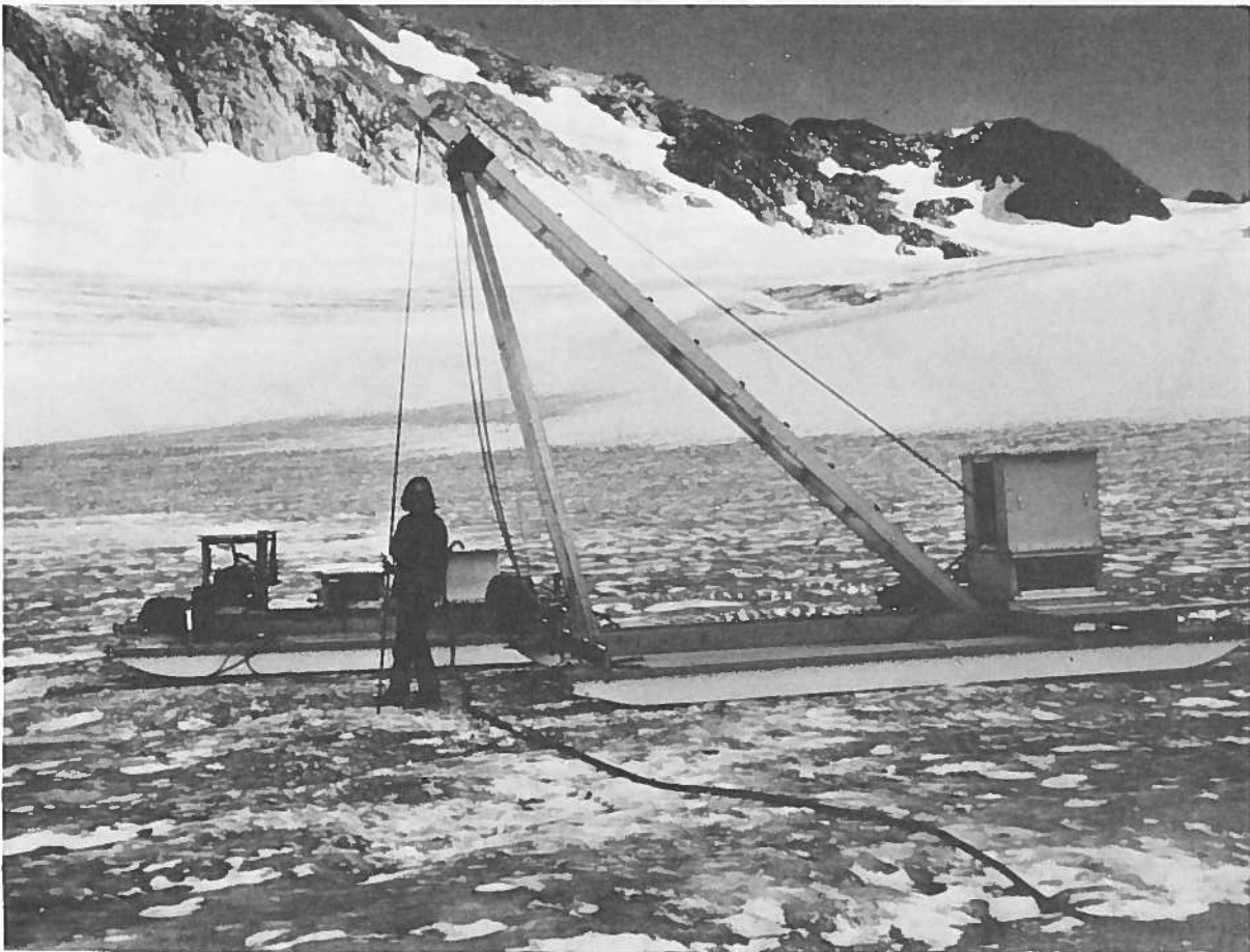
Figure 7. USGS Drill Sleds, South Cascade Glacier. Hose reel, winch drive, and boom sled in the foreground. Sled behind carries (right to left) the drill tank, electrically driven, high-pressure pump, water heater, and fuel tank. Operator is installing a hose spacer. Hose in the foreground brings water from a firn well near the previously drilled hole. Sleds are transported with a small track vehicle.
