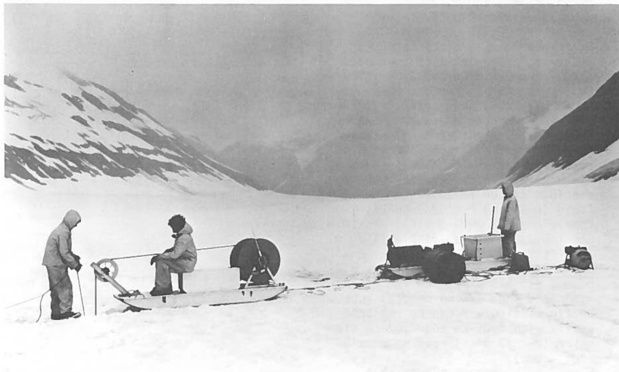
Figure 6. The Cal Tech sleds on Variegated Glacier, Alaska. Portable generator at the right, 55-gal fuel drum for the heater in the foreground. Gasoline engine-driven pump is behind the drum, between the tank and the heater. Hose reel, drive unit on the left sled. Operator on the far left is tending a cable to a pressure transducer down the same hole.
