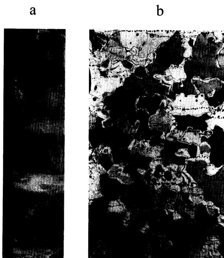
Fig. 1. Segment of the ice core taken with ATED (a) at T = -14^{\circ}\text{C} and (b) a vertical thin section ( 3.5 \times 2.5 cm) of an ice core obtained by a conventional thermal drill at T_i = -45^{\circ}\text{C} .
