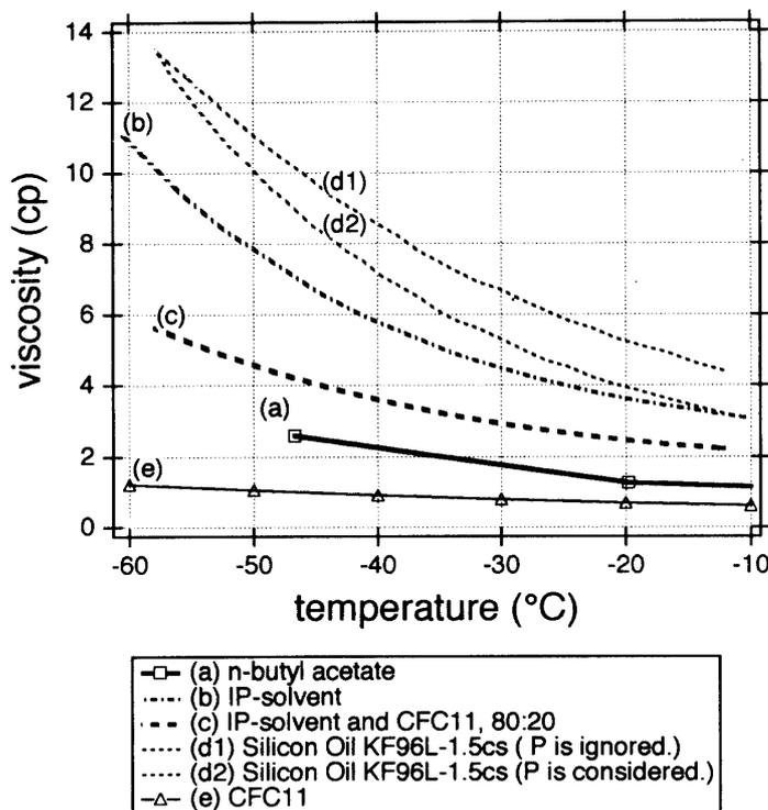
Fig. 6. The viscosity of the drilling fluid candidates. (a) is that of n-butyl acetate (GOSINK *et al.* 1991). (b) is that of IP-solvent measured by the authors. (c) is that of the mixture of IP-solvent and CFC11. These are calculated values based on (b) and (e). (d1) and (d2) are those of Silicone Oil, without and with the effect of hydrostatic pressure, respectively. (e) is that of CFC11.
