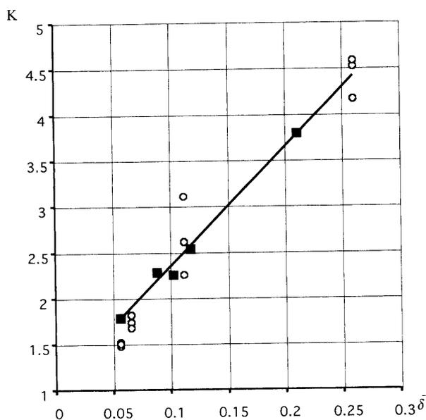
Fig. 2. Coefficient K versus relative clearance:
