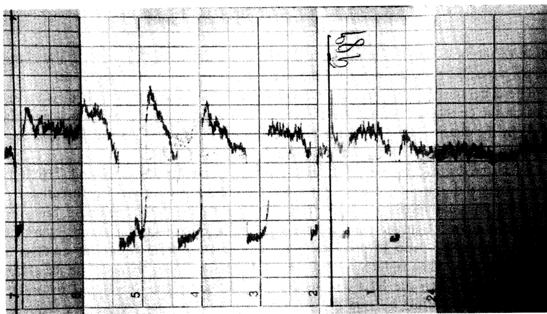
Fig. 2. Motor current for two runs. The right run is good, with only one cleaning, the left needed 4 times cleaning. Time goes from right to left.
