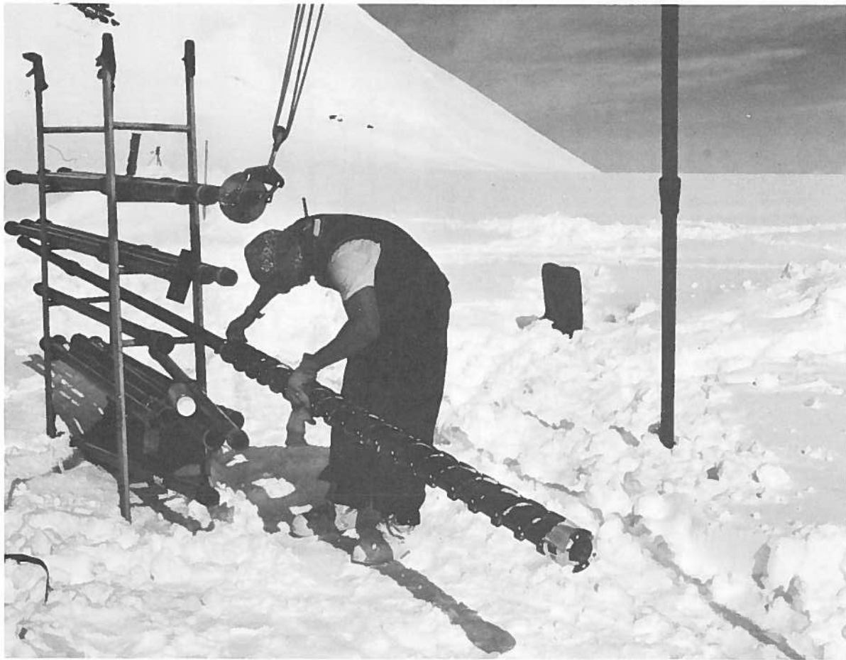
Figure 5. The 2 m auger barrel being prepared for another trip down the hole. The light weight of the PICO drill made it easy for one man to handle. The usefulness of the ladder as a rack for drill rods is especially apparent in this view. The base of the summit ridge is seen on the left of center.
