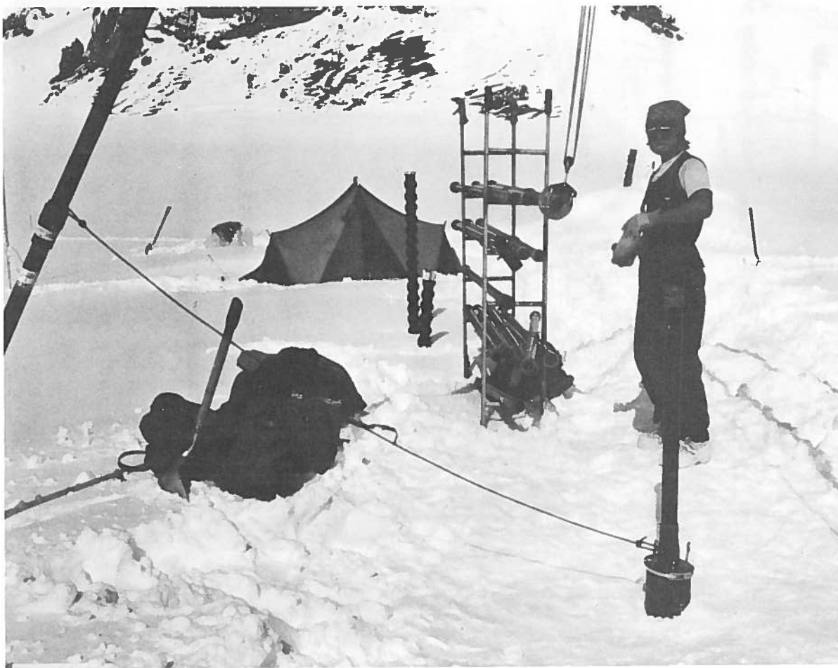
Figure 4. The 2 m auger barrel is shown being supported in the core hole by the support clamp on the casing, in order to protect it from direct solar radiation, while Dan prepares himself for the next drill run. The aluminum ladder, brought by helicopter from a cache on the rim of the North Crater, was very useful as a holder for drill rods.
