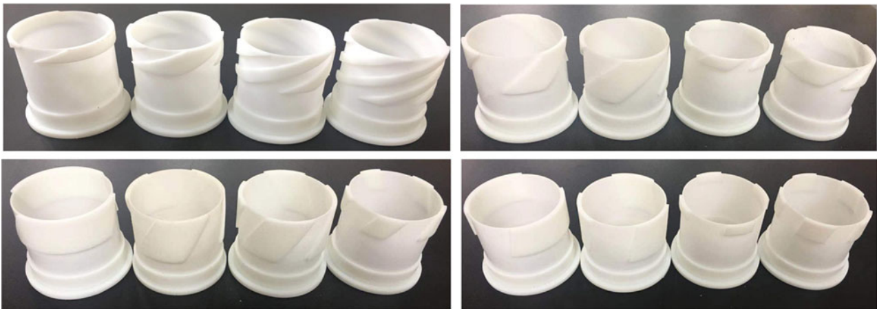
Fig. 6. Swirlers produced by 3D print technology.
