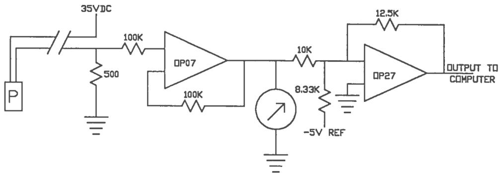
FIGURE 4. PRESSURE SENSING CIRCUIT.
