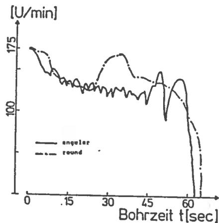
Fig. 2 - Recording of the cutter head rotation.
