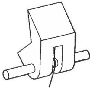
Figure 4 - Core catcher. The core catcher are pushed against the ice core with a small strong V-shaped wire spring. The catcher is prevented from falling into the head when not engaged using a soft spring placed in a groove in the catcher.
