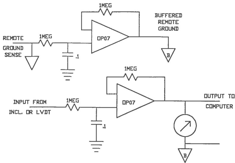
FIGURE 3. CIRCUIT DIAGRAM FOR SENSING REMOTE SIGNALS.
