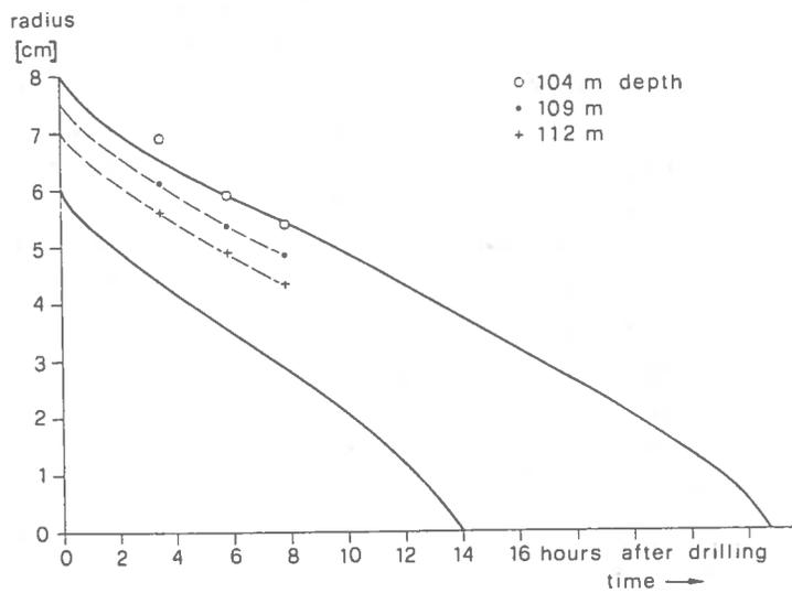
Fig. 11 - Calculated and measured freezing of boreholes at  $-12^{\circ}\text{C}$  (data from Fig. 10). The calculated hole radii (fat lines) refer to initial radii  $r_0 = 6$  and  $r_0 = 8$  cm, respectively.
