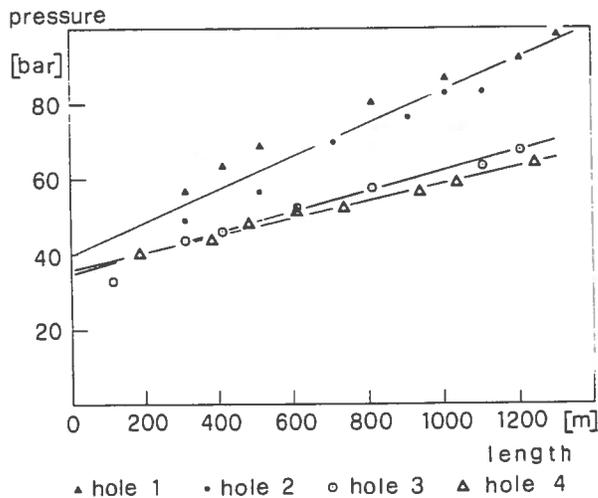
Fig. 6 - Applied pressure versus length of hose recorded during drilling with a discharge of 3.6 m<sup>3</sup>/h. At length 0 the pressure corresponds essentially to the loss of pressure head in the nozzle. Additional information is given in the text.
