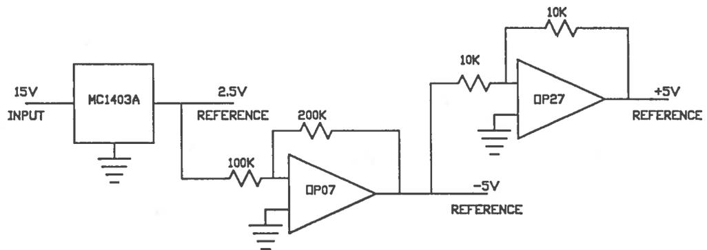
FIGURE 2. DIAGRAM OF VOLTAGE REFERENCE CIRCUIT.
