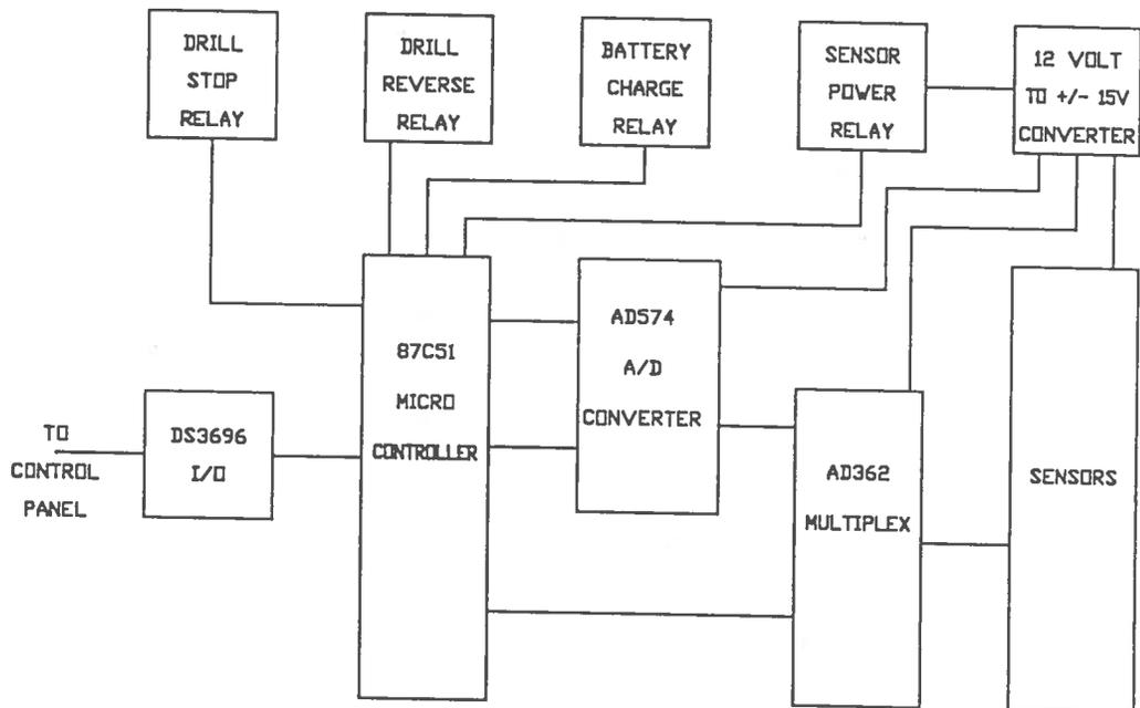
FIGURE 6. BLOCK DIAGRAM OF CIRCUIT IN ICE CORING DRILL
