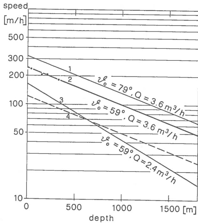
Fig. 5 - Drill speed as a function of depth assuming that R and C\* are constant. Data points correspond to the slope of the curve in Fig. 4.
