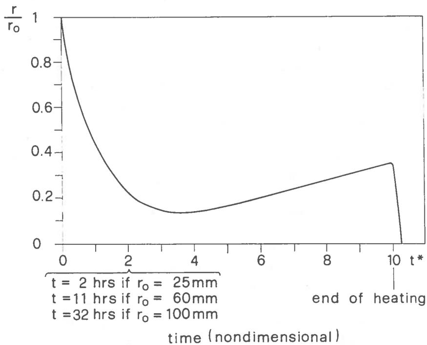
Fig. 13 - Calculated variation of hole radius due to slightly warm hose in hole. Ice temperature :  $-25^{\circ}\text{C}$ , assumed heat loss from hose :  $73 \text{ kcal}/(\text{mh}) = 85 \text{ Watt}/\text{m}$ .
