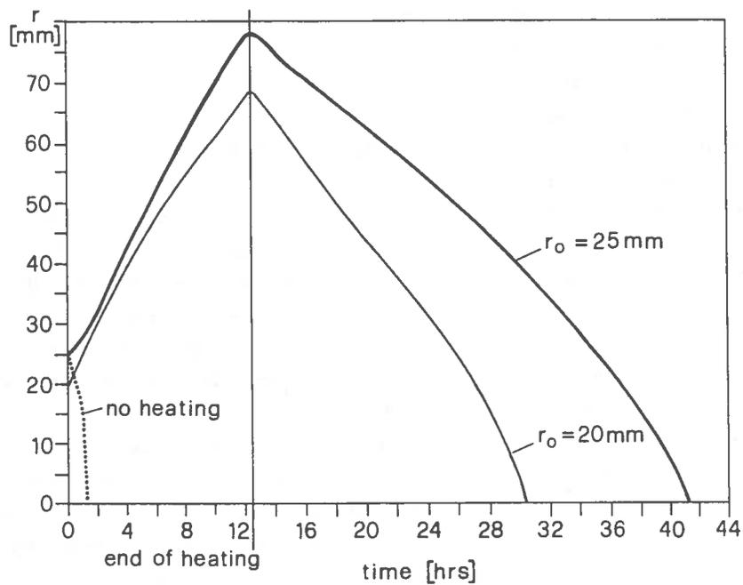
Fig. 12 - Calculated enlargement of a borehole after drilling by heat transfer from the drilling hose and subsequent freezing. Ice temperature :  $-20^{\circ}\text{C}$ , assumed heat loss from hose :  $150 \text{ kcal}/(\text{mh}) = 174 \text{ W}/\text{m}$ .
