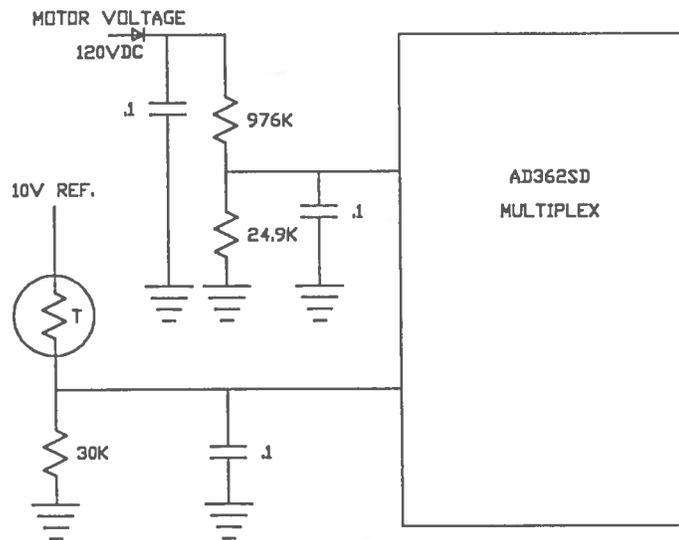
FIGURE 8. EXAMPLE OF SIMPLE CONDITIONING REQUIRED FOR SIGNALS
