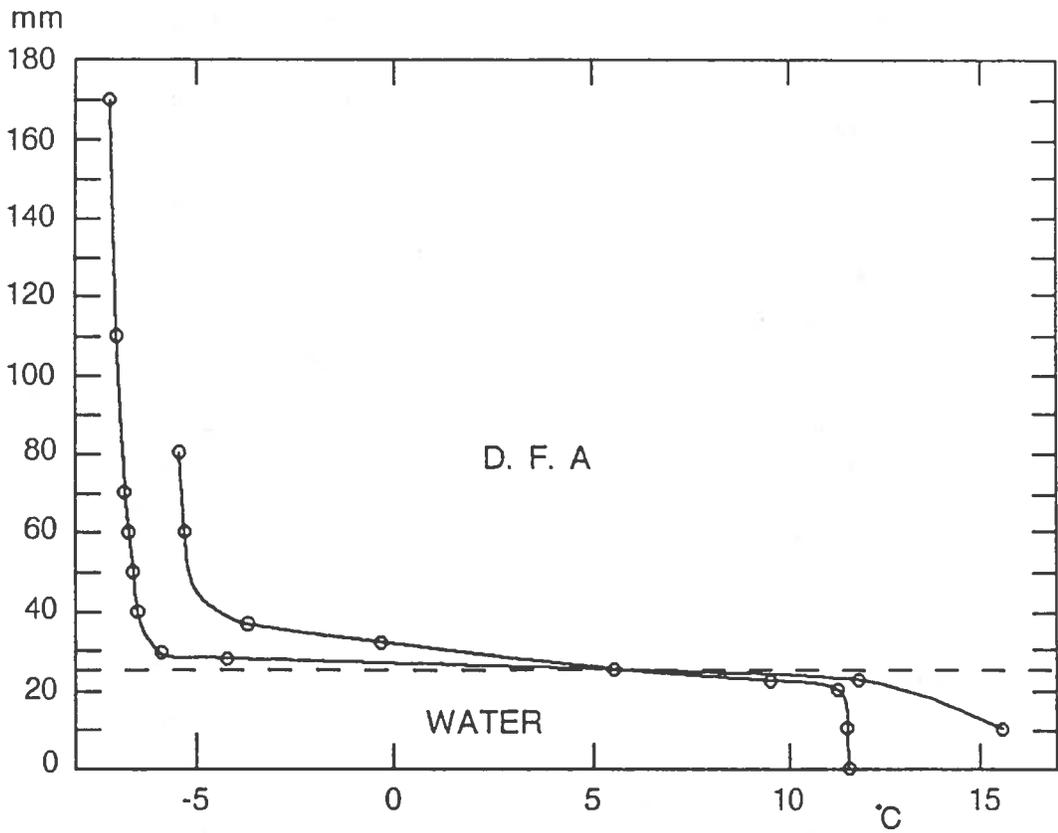
Fig.1 - Temperature profile at the water-DFA interface
