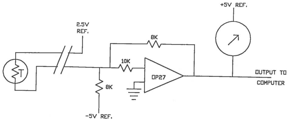
FIGURE 5. TEMPERATURE SENSING CIRCUIT
