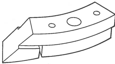
Figure 3 - Bits seen from above. The rake angle (the angle between vertical and the front plane of the cutter is  $45^\circ$ , the clearance angle is  $12^\circ$ . The bits are positioned with two pins, and held in place with a single screw.
