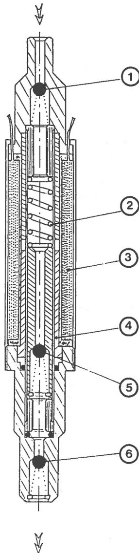
Fig. 2 Electromagnetic pump.
