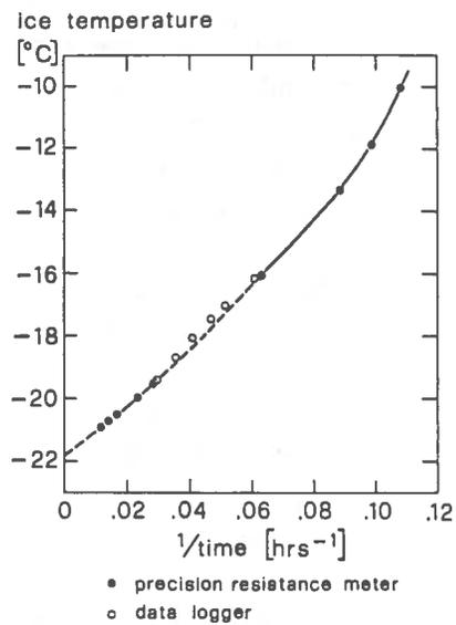
Fig. 7a - Temperature variation shortly after drilling. The thermistor is at 988 m depth. The thin, broken line sketches a typical temperature variation ; no measurements were taken during this time interval.
