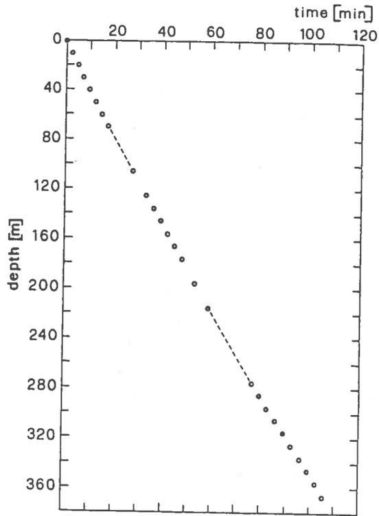
Fig. 4 - Depth of drill as a function of time in a test run. Nozzle diameter : 4 mm, discharge : 3.6 m<sup>3</sup>/h, water temperature at heater : 65°C.
