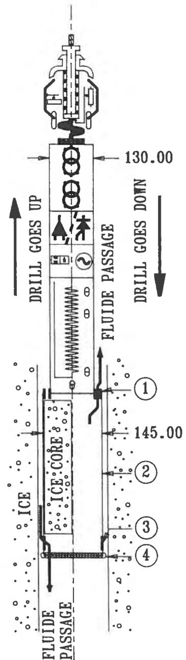
Figure 3 - Piston effect : Left part of the drawing : the drill goes up with the ice core inside the core barrel. Right part of the drawing : the drill goes down. (1) Four boring holes. (2) Core barrel section (see next paragraph). (3) Flap valve. (4) Piston effect zone.
