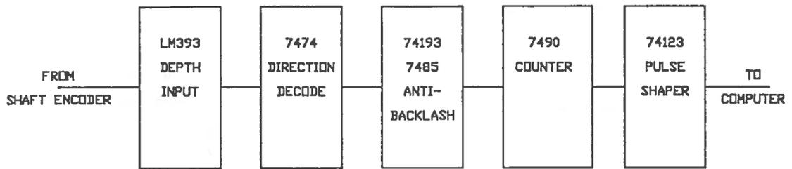
FIGURE 1. BLOCK DIAGRAM OF DEPTH RECORDING CIRCUIT.
