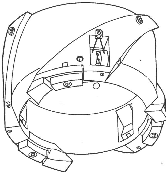
Figure 2 - Drill head as seen from below. On the inner surface, one corecatcher penetrates into the space for the ice core. Note, that the core catcher when not engaged do not fall down - a small soft spring between the core dog and the drill head prevents the dog to fall down. Also seen is the shoes mounted on the bits, after the cutting edge. The size of the shoe allow the handauger to start from the surface even in loose snow. The bits can be removed pushing a tool into a groove in the head.
