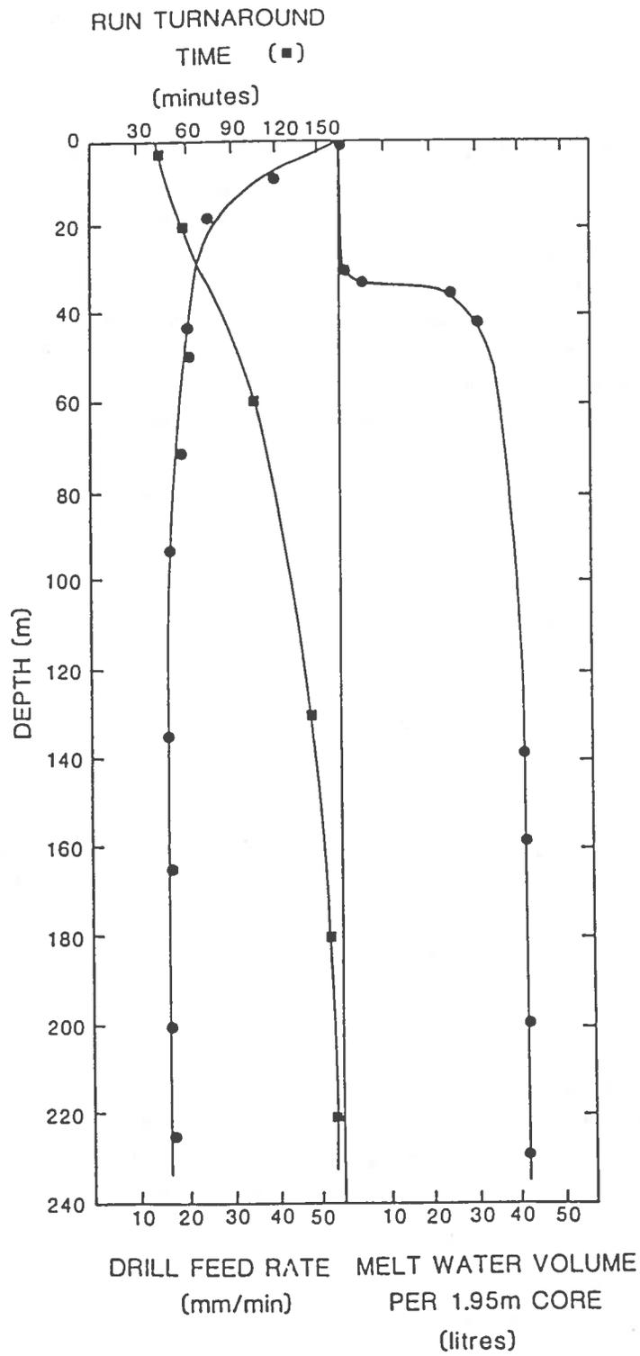
Figure 2 - Drill feed rate, run turn-around time (number of minutes per drilling run for a 1.95 metre core) and meltwater uptake.
