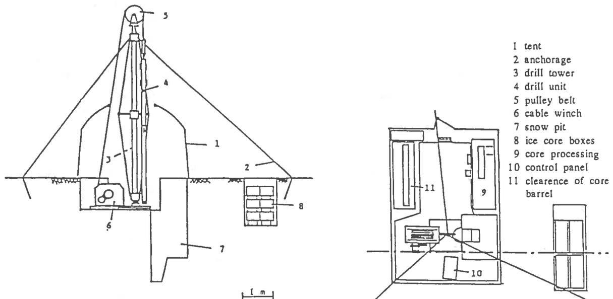
Fig. 1 - Arrangement of the drill equipment
