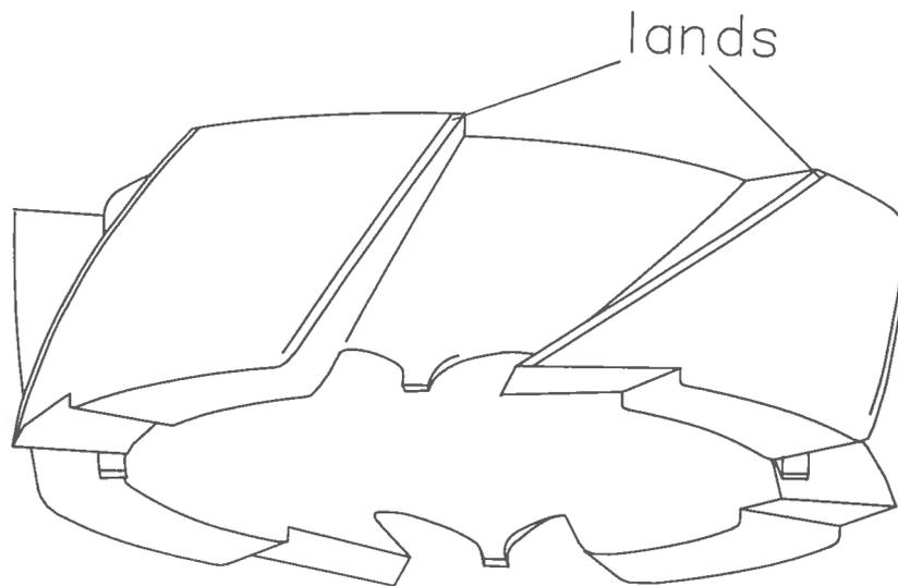
Fig. 2 - The new drill head. It is assembled of three rings (not shown). The cutters are integrated in the lowest ring. The core catchers are fixed to the central part and the upper ring is attached to the core barrel.
