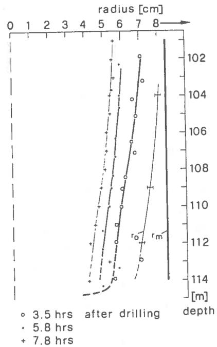
Fig. 10 - Gradual freezing of a borehole drilled to 114 m depth. Ice temperature at bottom of hole:  $-12^{\circ}\text{C}$ .
