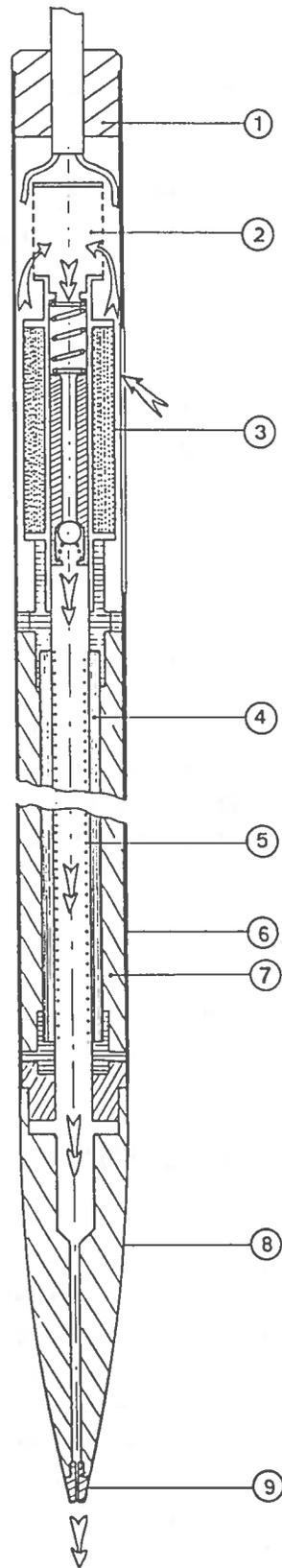
Fig. 1 Schematic diagram of the Electrochaude drill : (1) Cable anchorage ; (2) Filter ; (3) Electromagnetic pump ; (4) Ceramic tube ; (5) Heating wire ; (6) Stainless steel external tube ; (7) Weight ; (8) Nozzle ; (9) Tip.
